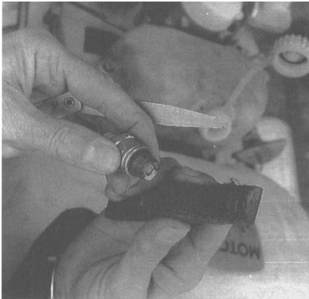
Fig. 15.3 Cleaning spark plug and checking gap.
