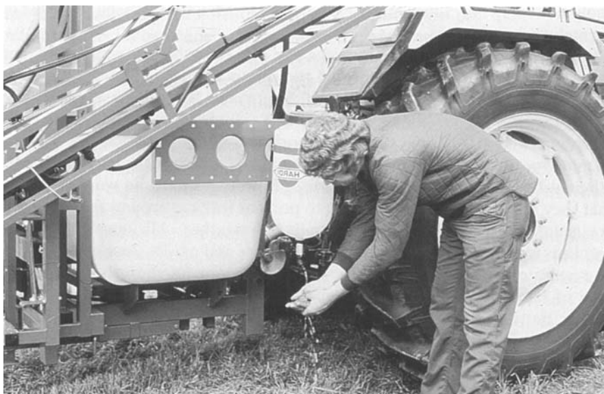
Fig. 16.3 Using extra clean water tank on sprayer to wash hands.
