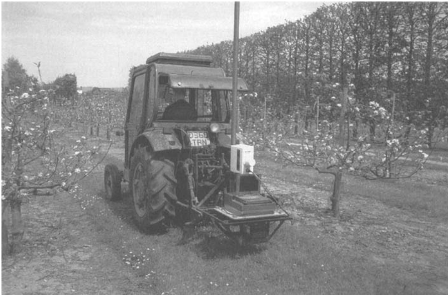
Fig. 10.18 (a) measurements of crop to calibrate sprayer application rate. (b) LIDAR equipment to assess tree canopy.
