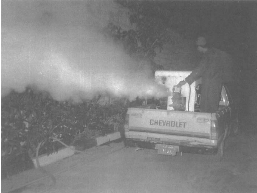
Fig. 11.6 TIFA fogger mounted on vehicle.
