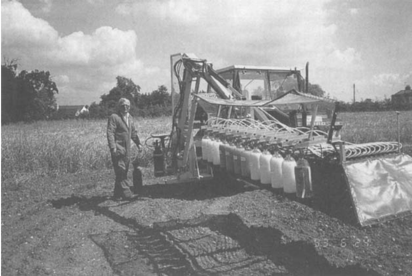
Fig. 18.6 Plot sprayer made by adaptation of tractor-mounted hedgecutter. Note individual containers of pesticide for each plot (photo: J.H. Crabtree).
