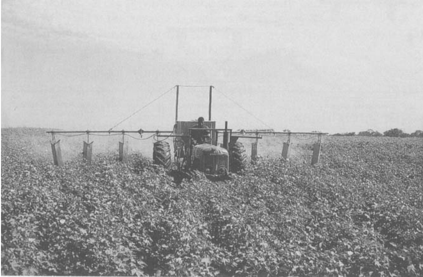
Fig. 7.15 Tractor sprayer with vertical booms between row crop.
