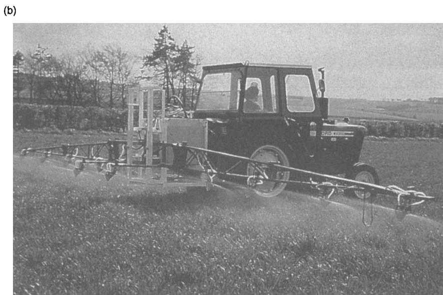
Fig. 8.12 (a) Spinning nozzle for use on tractor. (b) Tractor boom fitted with Micromax nozzles.
