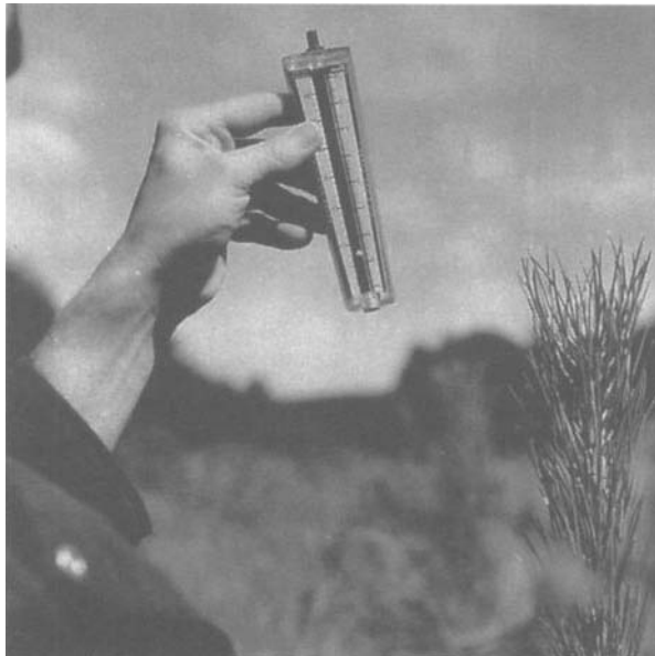
Fig. 8.7 Measuring wind velocity with a simple anemometer.
