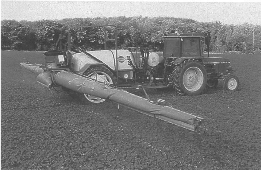
Fig. 10.13 (a) Diagram to show relative position of airflow from airsleeve and spray from nozzle. (b) Air-sleeve sprayer.
