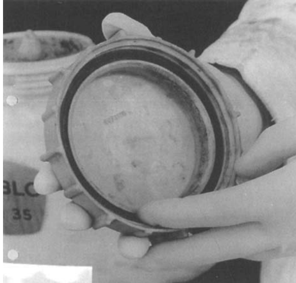
Fig. 15.2 Checking seal on lid of spray tank of motorized knapsack mistblower.
