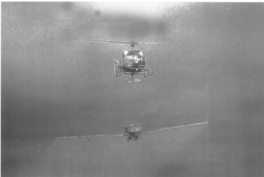
Fig. 13.8 Underslung unit on helicopter (photo: Simplex).
