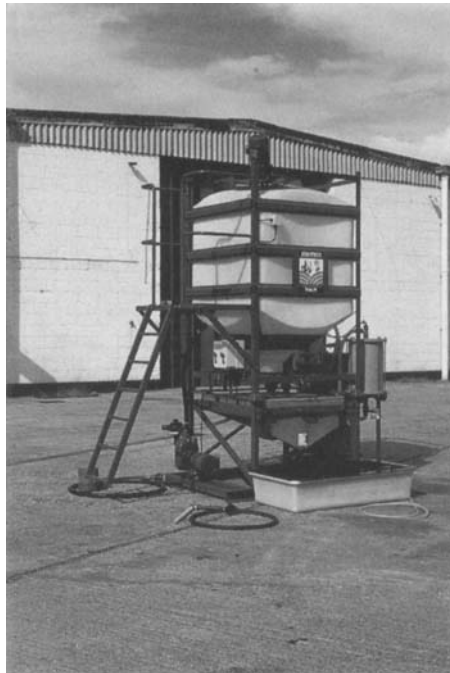
Fig. 16.6 'Sentinel' system for decontaminating water used to wash sprayers and containers.
