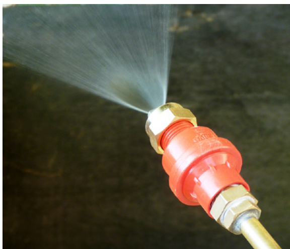
Figure 6.3 Close-up of fan nozzle with control flow valve. Reproduced with permission from Global Agricultural Technology & Engineering - GATE LLC. For a colour version of this figure, please see Plate 6.1.
