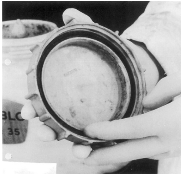
Figure 17.2 Checking the seal on the lid of the spray tank of a motorised mistblower. Photo: F. Wright.
