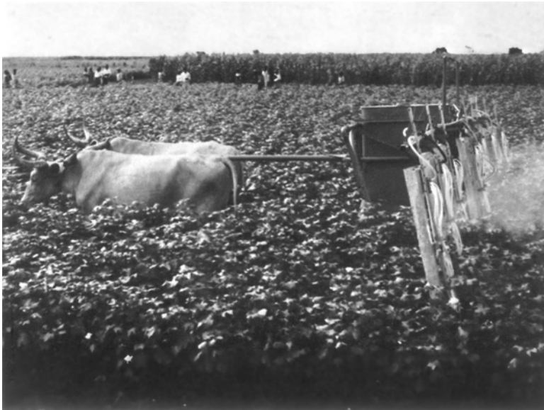
Figure 7.26 Animal-drawn sprayer with engine-driven pump.
