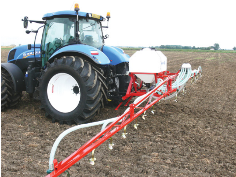
Figure 13.8 (a) Front-mounted Avadex granule applicator. (b) Rear-mounted 12 m granule applicator. (a) and (b) courtesy of Techneat Engineering Ltd.
