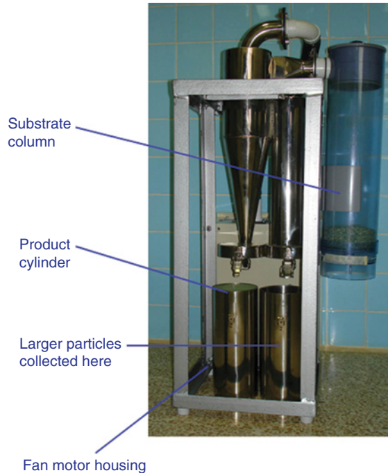
Figure 16.2 The MycoHarvester v.5 extracting fungal conidia from a grain substrate. Courtesy of MycoHarvester.
