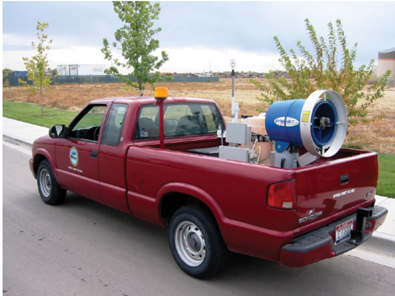
Plate 14.2 Truck-mounted cold fogger fitted with GPS and mini meteorological station. (Courtesy of New Mountain Innovations Inc.)
