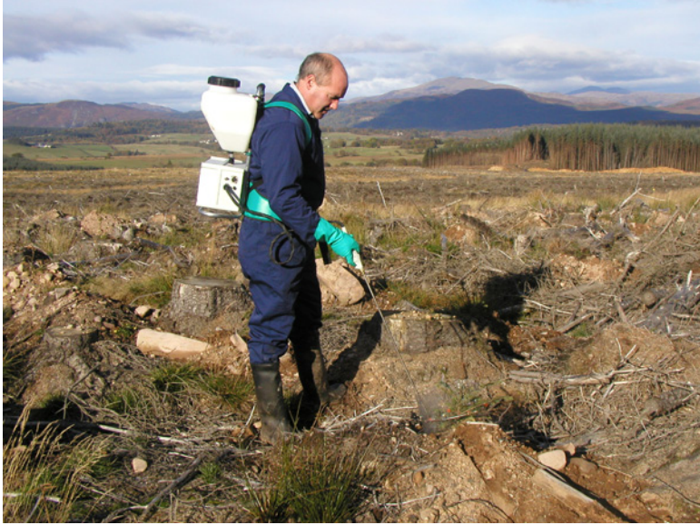
Figure 6.6 Autos electrically operated knapsack sprayer used to apply a fixed volume per tree. Courtesy of Micron Sprayers Ltd. For a colour version of this figure, please see Plate 6.2.
