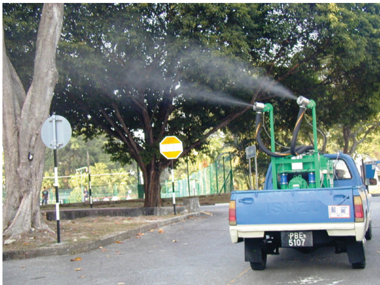
Plate 14.1 Vehicle-mounted cold fogger used for mosquito control. (Courtesy of Micron Sprayers Ltd.)
