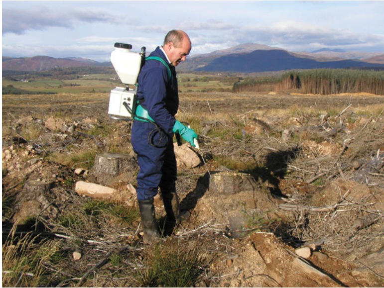
Plate 6.2 Autodos electrically operated knapsack sprayer used to apply a fixed volume per tree. Courtesy of Micron Sprayers Ltd.
