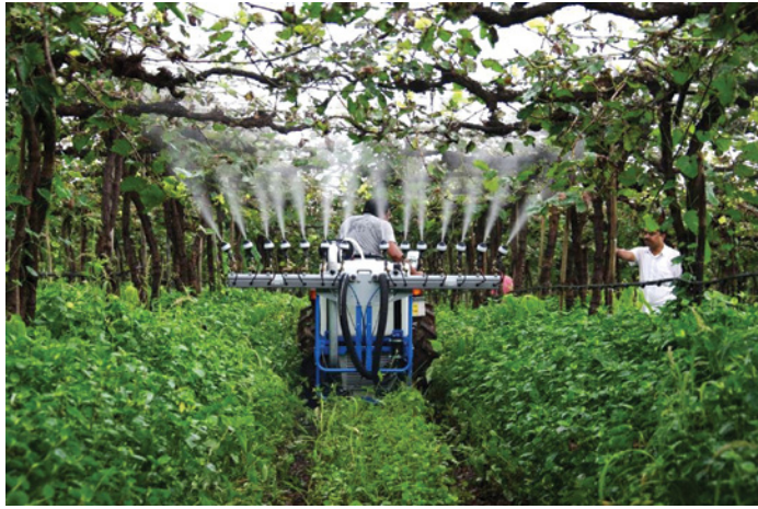
Plate 10.1 Electrostatic sprayer treating vines in India. Courtesy of Edward Law.
