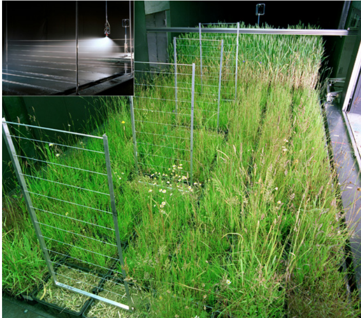
Figure 12.5 Passive sampling lines 2.0 mm in diameter sampling airborne spray in wind tunnel experiments. Courtesy of NIAB-TAG. For a colour version of this figure, please see Plate 12.2.
