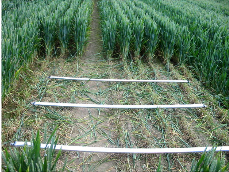
Figure 12.4 Sampling laths supporting chromatography paper for measuring sedimenting spray downwind of a treated crop area. (Photo courtesy of NIAB-TAG.)
