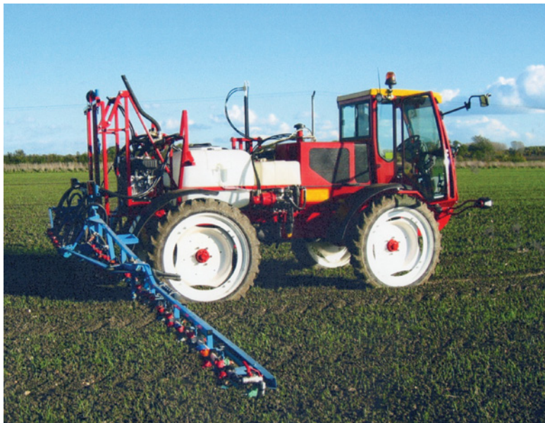
Plate 19.1 Agribuggy showing the 500L clean water tank with smaller 250L waste tank for plot spraying. (Courtesy of Tom Robinson at Syngenta UK Limited.)
