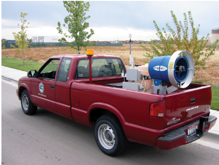
Figure 14.10 (a) Truck-mounted cold fogger fitted with GPS and mini meteorological station. (b) Close-up of meteorological sensor. (a) and (b) courtesy of New Mountain Innovations Inc. For a colour version of part (a), please see Plate 14.2.
