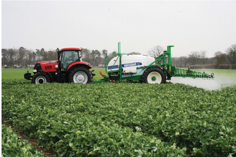
Plate 7.1 Various types of power-operated hydraulic sprayers. Tractor trailed sprayer. Courtesy of Househam Sprayers Ltd.
