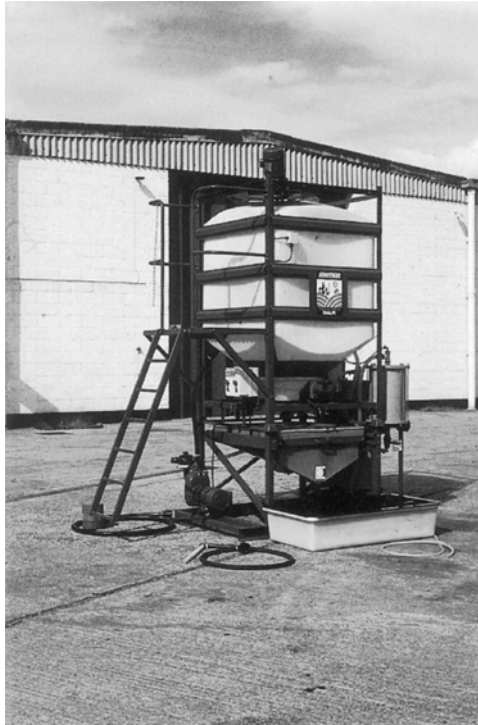
Figure 18.6 'Sentinel' system for decontaminating water used to wash sprayers and containers.
