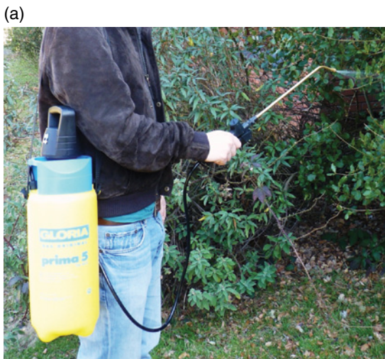
Figure 6.8 Battery-operated compression sprayer, (a) showing sprayer being used and (b) the pump in which batteries are fitted.
