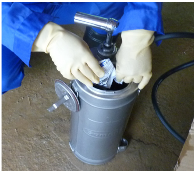
Figure 3.6 Emptying a sachet of insecticide into a compression sprayer. For a colour version of this figure, please see Plate 3.1.
