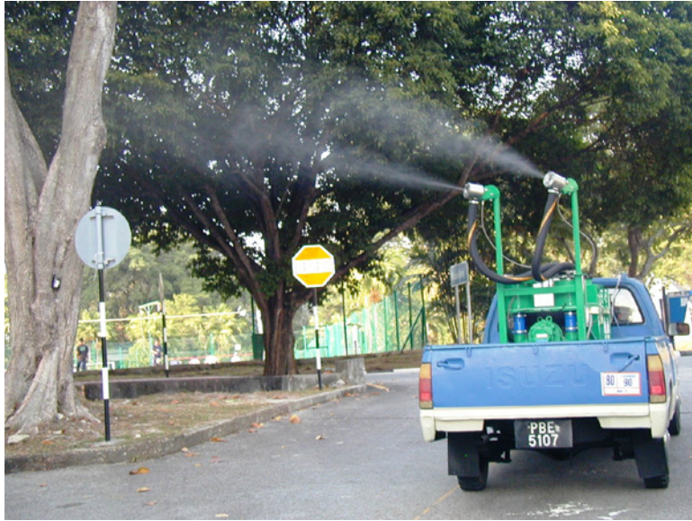
Figure 14.9 Vehicle-mounted cold fogger used for mosquito control. Courtesy of Micron Sprayers Ltd. For a colour version of this figure, please see Plate 14.1.
