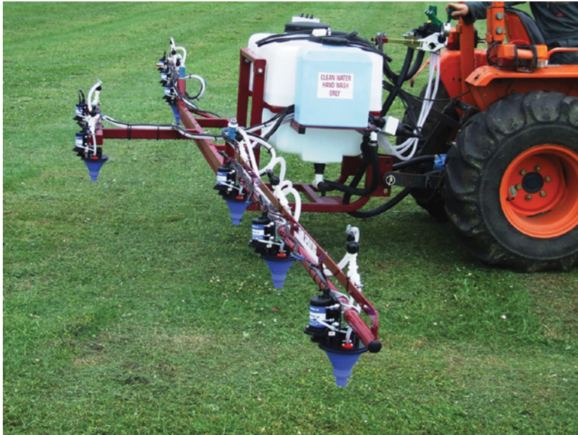
Figure 9.14 (a) Micromax unit. (b)Tractor boom fitted with Micromax nozzles. (a) and (b) courtesy of Micron Sprayers Ltd.
