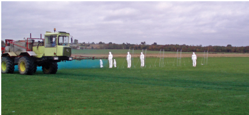
Plate 12.1 A typical field drift trial measuring sedimenting and airborne spray at different distances downwind of a spray track together with deposits on bystanders. (Courtesy of NIAB-TAG.)
