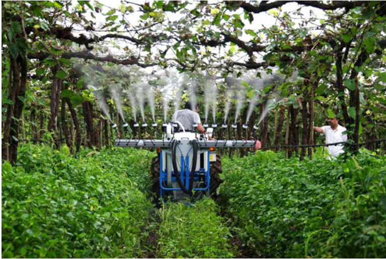
Figure 10.10 Electrostatic sprayer treating vines in India. Courtesy of Edward Law. For a colour version of this figure, please see Plate 10.1.
