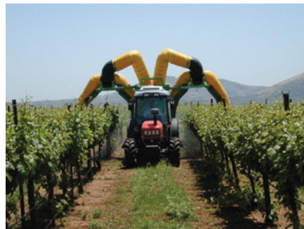
Figure 8.16 Orchard sprayers. (a) With axial fan. (b) With ducting over axial fan. (c) With cross-flow fan. (d) With centrifugal fan. (e) With 'Turbocoll' system. (f) Eagle sprayer in vineyard. Courtesy of Degania Sprayers.
