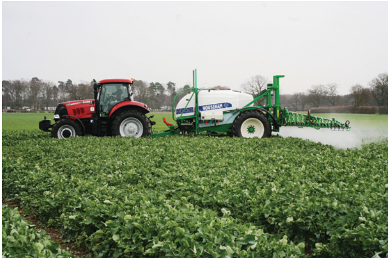
Figure 7.1 Various types of power-operated hydraulic sprayers. (a) Mounted on three-point linkage to tractor. (b) Tractor trailed sprayer. (c) Trailed sprayer. (d) Self-propelled sprayer. Photos (b), (c) and (d) courtesy of Househam Sprayers Ltd. For a colour version of part (b), please see Plate 7.1.
