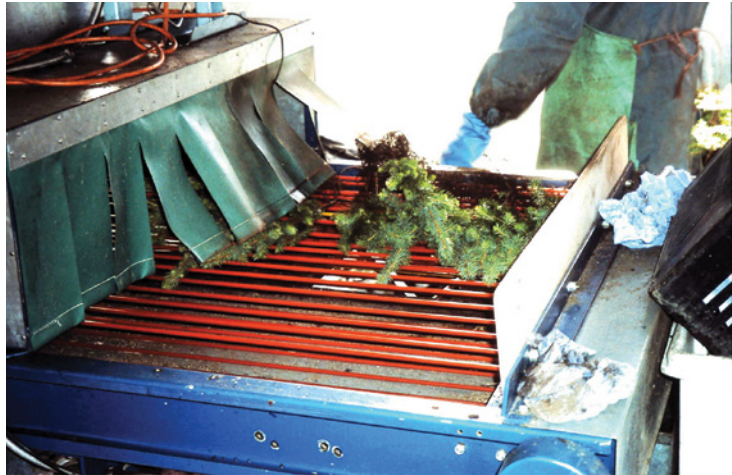
Figure 10.11 Electrostatic spraying of tree seedlings prior to planting, with an Electrodyn sprayer. (a) Spraying plants. (b) Loading conveyor system. (c) Removing treated plants.
