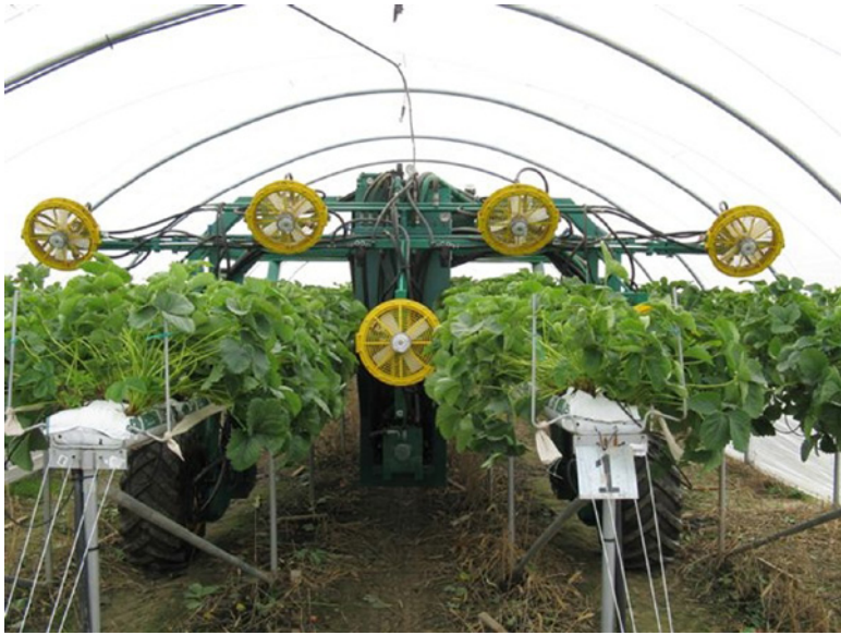
Figure 8.18 Air-assisted sprayer in polytunnel spraying strawberries. Courtesy of Micron Sprayers Ltd.
