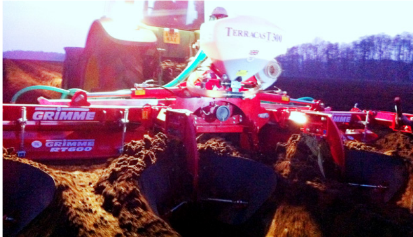
Figure 13.9 Terracast 300 nematicide applicator on a bed former. Courtesy of Techneat Engineering Ltd.
