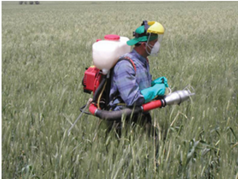
Plate 8.1 Motorised knapsack mistblower with rotary nozzle. Courtesy of Micron Sprayers Ltd.
