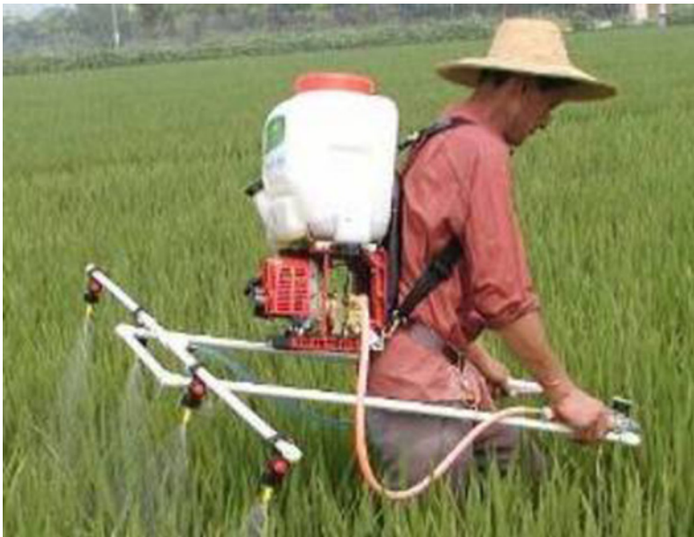
Figure 6.7 Motorised knapsack sprayer with two-stroke engine. Reproduced from Xiongkui He (2010). Courtesy of Xiongkui He.
