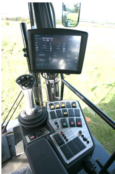
Figure 7.2 Sprayer controls in tractor cab including GPS. Courtesy of Househam Sprayers Ltd.
