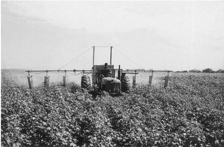
Figure 7.16 Tractor sprayer with vertical booms between the rows.
