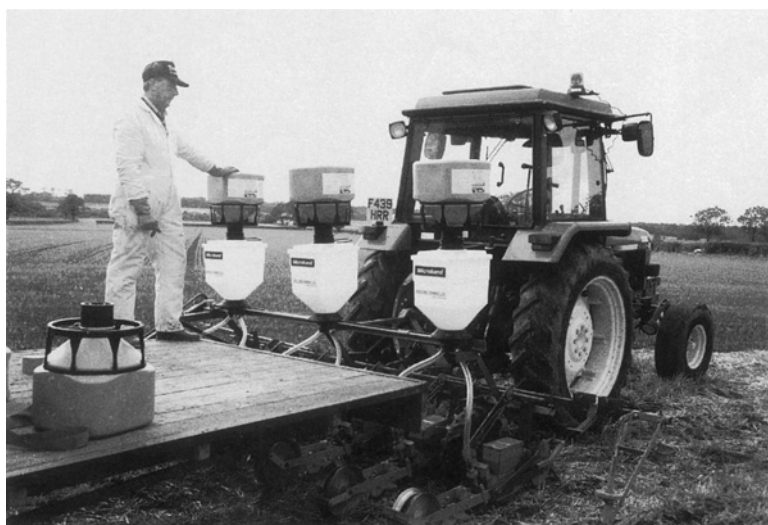
Figure 13.12 'Sure-Fill' closed granule transfer system. Photo: Horstine Farmery.
