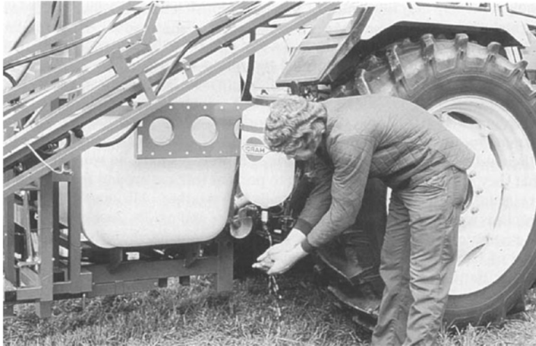
Figure 18.3 Using extra clean water tank on sprayer to wash hands. Photo: Allman.
