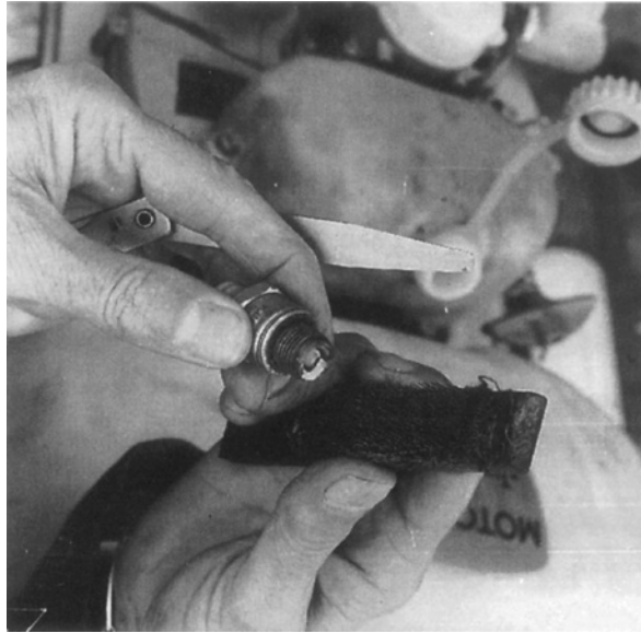
Figure 17.3 Cleaning the spark plug and checking the gap. Photo: F. Wright.
