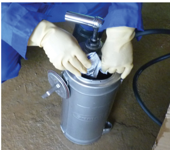
Plate 3.1 Emptying a sachet of insecticide into a compression sprayer.
