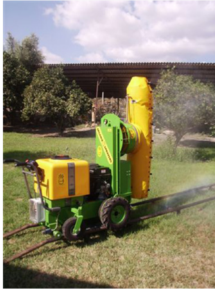
Figure 8.14 Small unit with air sleeve to provide airflow to project spray. Courtesy of Degania Sprayers.
