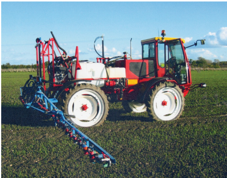
Figure 19.7 (a) Agribuggy with 60 litre spray tank and 12 m recirculating boom with four nozzle turrets at 50 and 25 cm spacing. (b) Agribuggy showing the 500 L clean water tank with smaller 250 L waste tank for plot spraying. (a) and (b) courtesy of Tom Robinson at Syngenta UK Limited. For a colour version of part (b), please see Plate 19.1.
