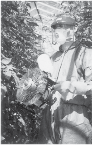
Figure 9.11 (a) Electrafan 12 sprayer. (b) Electrafan being used in a glasshouse. (c) Motorfan sprayer with two-stroke engine being used in a glasshouse. (d) Flying Doctor multiple Electrafan units in a glasshouse. All photos courtesy of Micron Sprayers Ltd.
