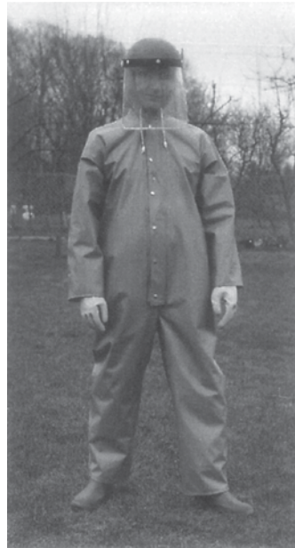
Figure 18.2 Protective clothing. (a) Extra protection spun-bonded polypropylene coverall. Breathable, so no permeation resistance; hence the need for an impermeable apron. Faceshield used when handling concentrates. (b) Polyethylene-coated spun-bonded polypropylene coverall. Not breathable, but low resistance to permeation. (c) Tyvek coverall (spun-bonded polyethylene). Not breathable. Fairly high permeation resistance. (d) PVC-coated nylon coverall. Not breathable. High resistance to permeation. Apron not needed but protect coverall before entering tractor cab. Photos: MAFF CSL.
