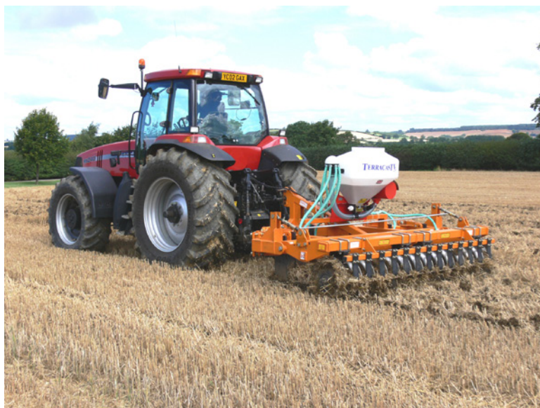
Figure 13.11 Terracast rape seeder with granule applicator. Courtesy of Techneat Engineering Ltd. For a colour version of this figure, please see Plate 13.1.
