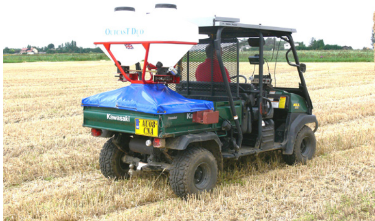
Figure 13.10 Outcast Duo Slug pelleter, 24m spread, mounted on a utility vehicle. Courtesy of Techneat Engineering Ltd.
