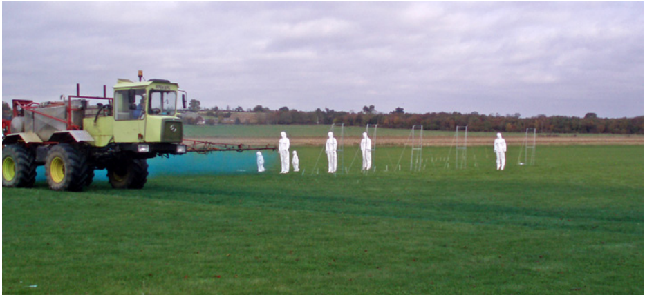
Figure 12.3 A typical field drift trial measuring sedimenting and airborne spray at different distances downwind of a spray track together with deposits on bystanders. Courtesy of NIAB-TAG. For a colour version of this figure, please see Plate 12.1.
