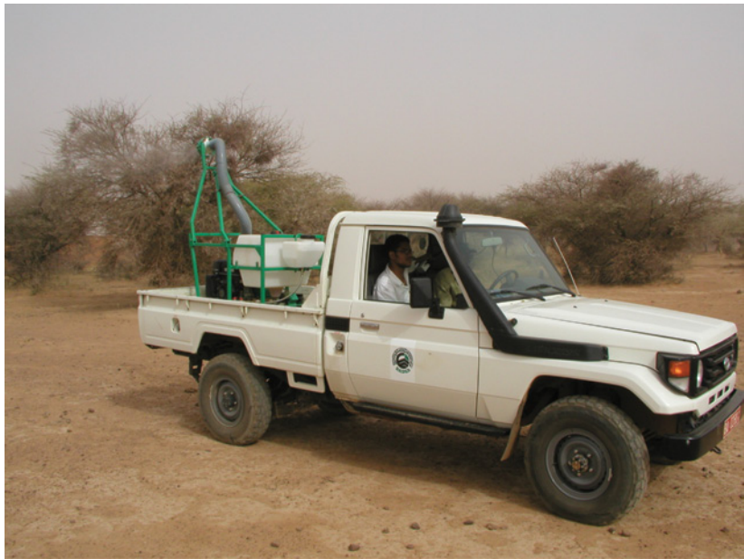
Plate 2.1 Locust control. Spinning disc sprayer ('ULVA mast') being used to control locusts. Courtesy of Micron Sprayers Ltd.
