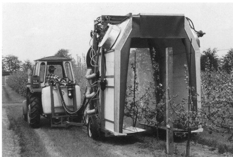
Figure 8.17 Tunnel sprayer. Photo: G. Doruchowski.
