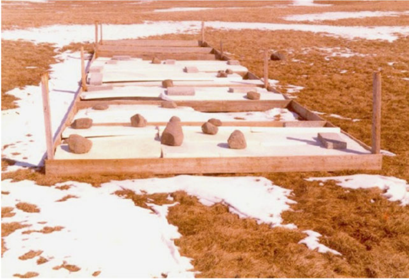
Fig. 4 Ice cover protected with styrofoam in a provocation test in Iceland in early spring 1979 (B.E. Gudleifsson)
