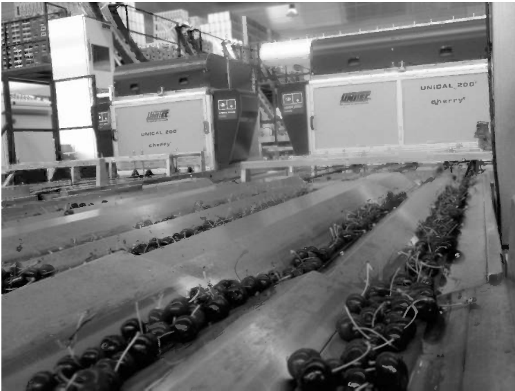
Figure 10.3 High-speed colour and defect sorting of cherries
