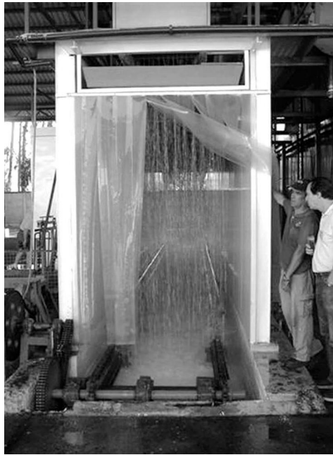
Figure 4.5 Hydrocooling unit designed to remove field heat from harvested stone fruit in bulk plastic bins. The bins travel slowly through a high-volume cold water shower. Cooling fruit from about 35°C to about 18°C takes approximately 20 minutes.
