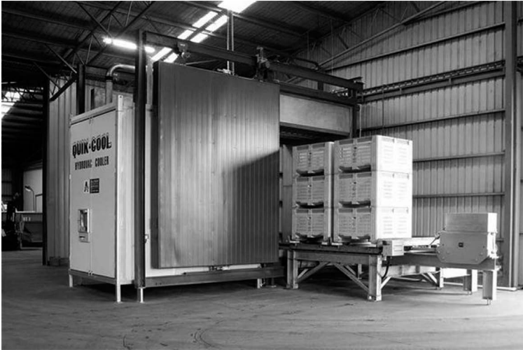
Figure 4.6 Hydro-vacuum cooler with capacity to cool four pallets of produce
