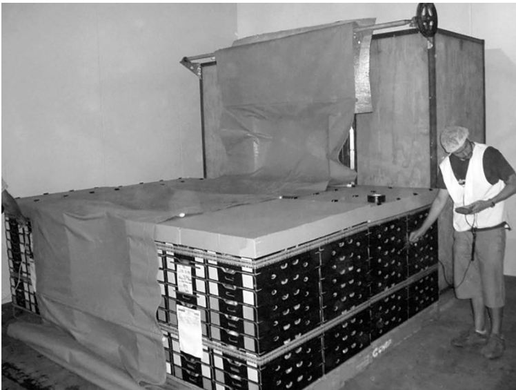
Figure 4.4 Air flow in forced-air (pressure) cooling. Packages and containers must be vented (at least 5% of exposed surface area) and stacked so that the cooling air is forced to flow through the containers and around the produce to return to the exhaust fans. A slight pressure drop occurs across the produce as air exhausts from the space between the stacks of produce.
