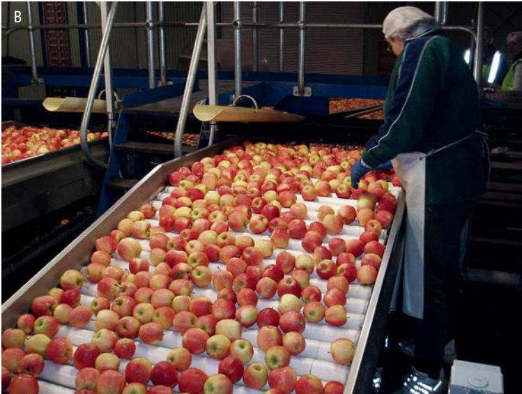
Plate 6 Transfer of apples through the packing line in sanitised water (A) and on rollers (B)
