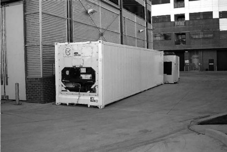
Figure 7.7 Insulated shipping container fitted with a built-in refrigeration unit
