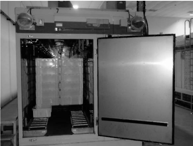
Figure 11.9 Commercial vapour heat treatment unit used to disinfest mango fruit
