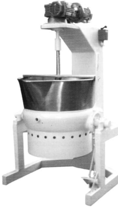
Fig. 11.8 Open pan with gas cooking facility and with mixer, used for the manufacture of jams and jellies (courtesy of Incal).
