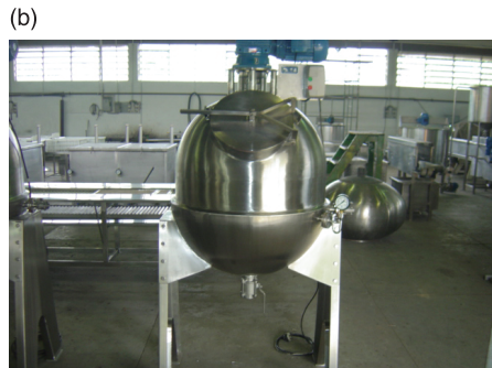
Plate XV (Chapter 11) Steam jacketed pans used in jams and jellies manufacture concentration. (a) Open steam jacketed pan with mechanical stirrer and (b) vacuum pan concentrator ('Buller') (courtesy of Mecamau).
