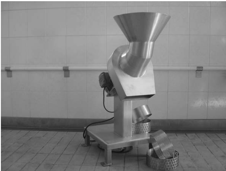
Fig. 11.1 Mill knife used to crumble fruit for juice extractor (courtesy of Mecamau).
