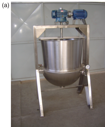
Plate XV (Chapter 11) Steam jacketed pans used in jams and jellies manufacture concentration. (a) Open steam jacketed pan with mechanical stirrer and (b) vacuum pan concentrator ('Buller') (courtesy of Mecamau).
