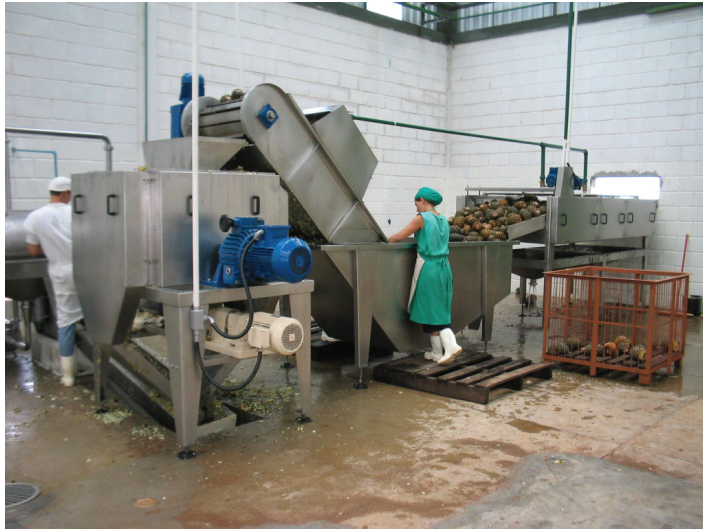
Plate XIV (Chapter 11) Line for pineapple juice extraction (courtesy of Tropical Food Machinery).
