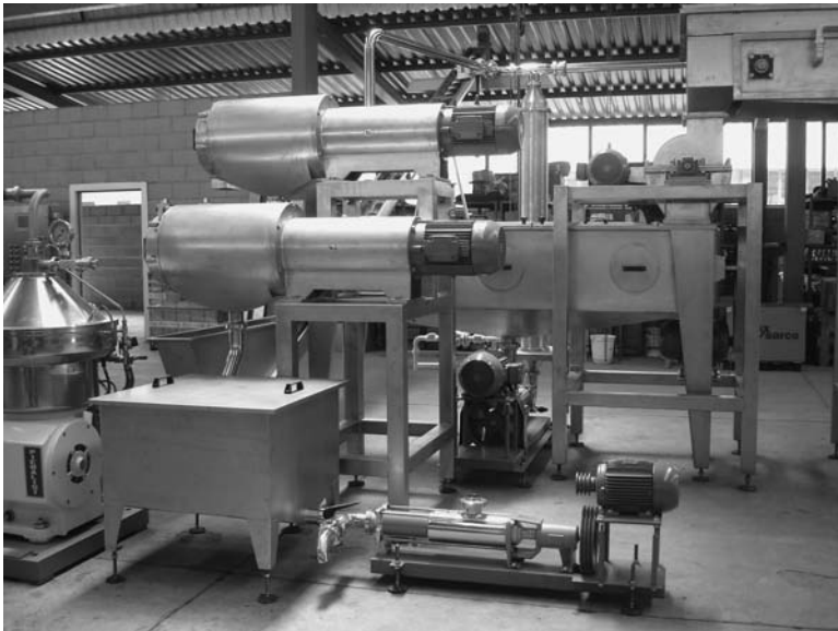
Fig. 11.2 Double fruit juice extractor (courtesy of Tropical Food Machinery).
