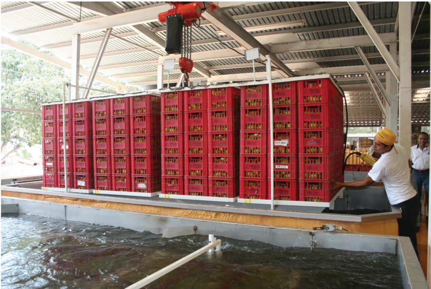
Plate II (Preface) Hot water treatment for quarantine insect control of mango in Mexico.
