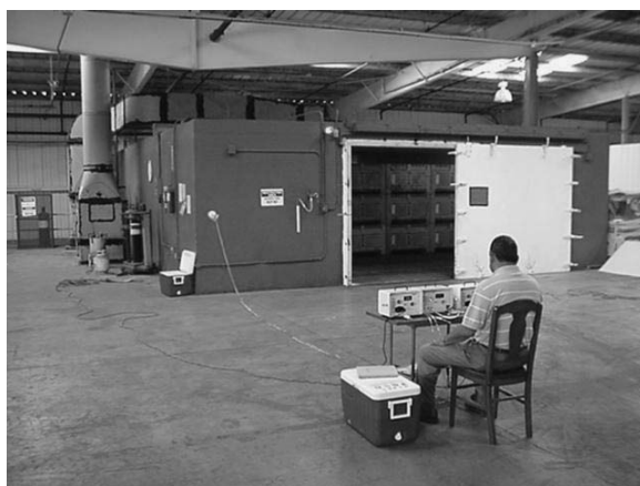
Fig. 7.3 Methyl bromide fumigation chamber at Edinburg, Texas (courtesy of USDA).
