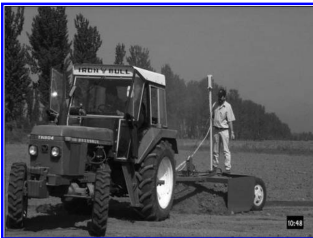
FIGURE 8.31 Land leveler in operation.
