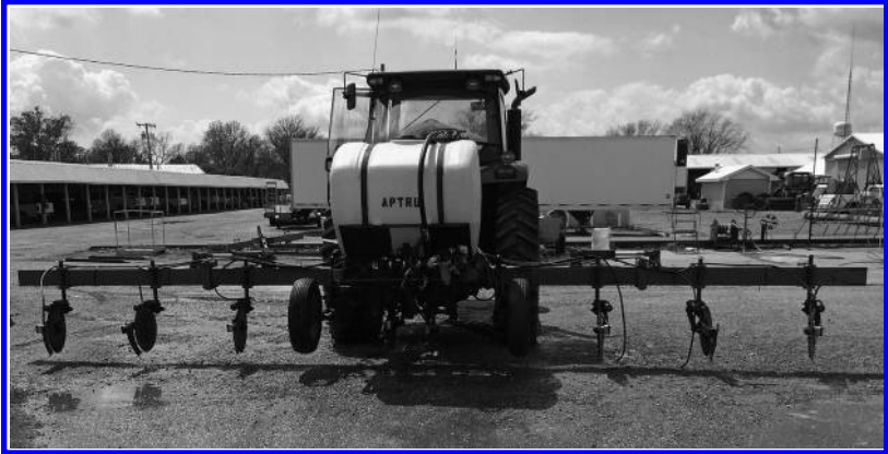
FIGURE 6.1 A map-based variable-rate liquid fertilizer applicator. Prescription maps can be uploaded and displayed in the controller installed inside the cab.
