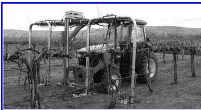
FIGURE 4.15 A robotic target sprayer for vineyard pest control. It can use less than 10% of pesticides to achieve similar efficacy with certain pest control compared to conventional broadcast applications.
