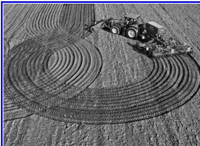
FIGURE 5.13 John Deere’s iTEC Pro for hands-free turns and implement control at headlands. (Photo courtesy of Deere & Company.)
