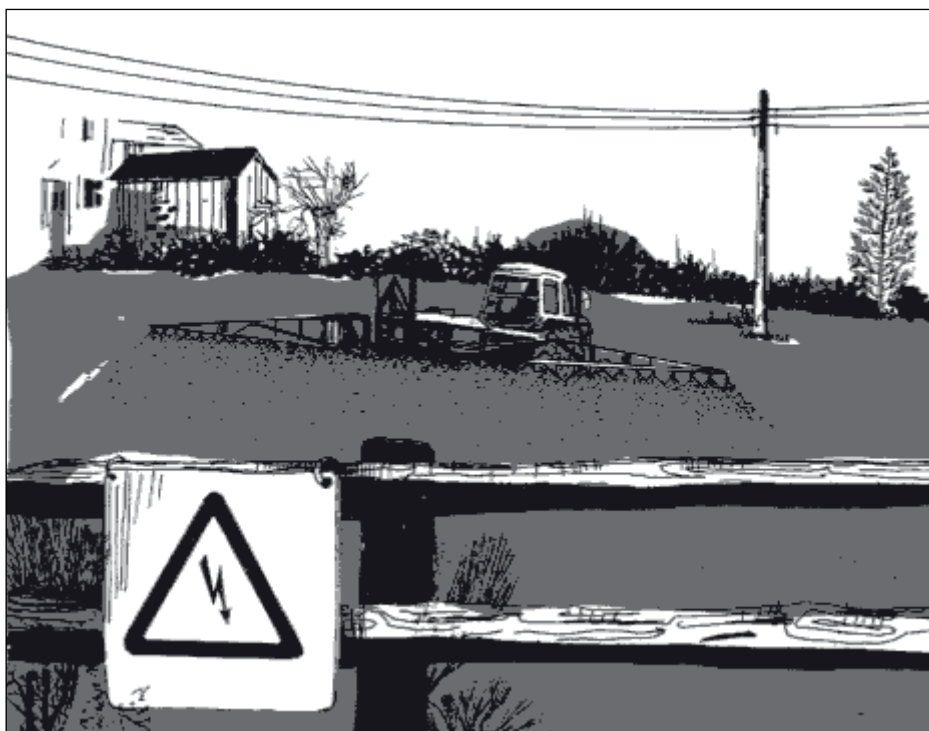
Figure 19. Look out for overhead electricity cables
