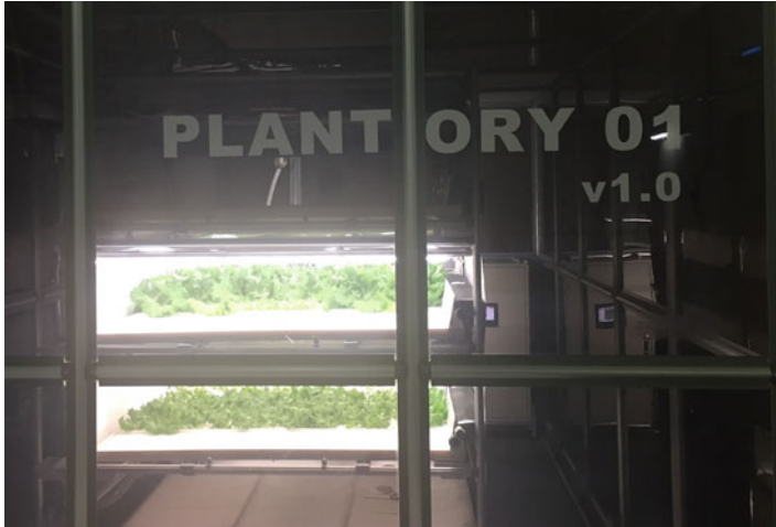
Fig. 5.26 The cultivation rack with four tiers is in an airtight plastic-covered room consisting of a CSM (Type A), developed by PlantX Corporation. This CSM can also be used as four Type B-a CSMs if the environmental factors at the inlet and outlet are measured for each tier
