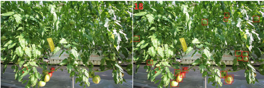
Fig. 23.7 Example of tomato detection and counting (note: green, red, and overlapped tomatoes are all counted)
