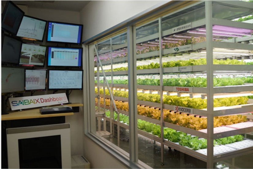
Fig. 9.11 Large-scale commercial-use PFAL and SAIBAIX dashboard (LCD display on left side of photo). Cultivation trials using LED lighting equipment from various manufacturers are being carried out in the cultivation chamber. (Chiba University Kashiwa no Ha Campus, Japan)
