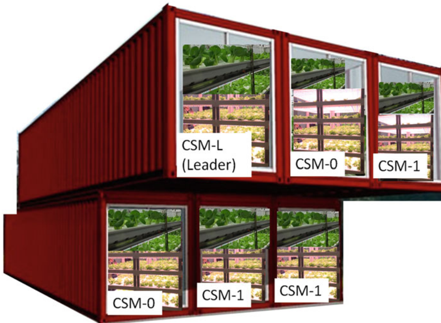
Fig. 5.27 Image of CSMs (Type A or Type B-a) that do not use a cultivation rack in the cultivation room. The distance between the CSMs is changeable. This CSM can be used for either Type A or Type B
