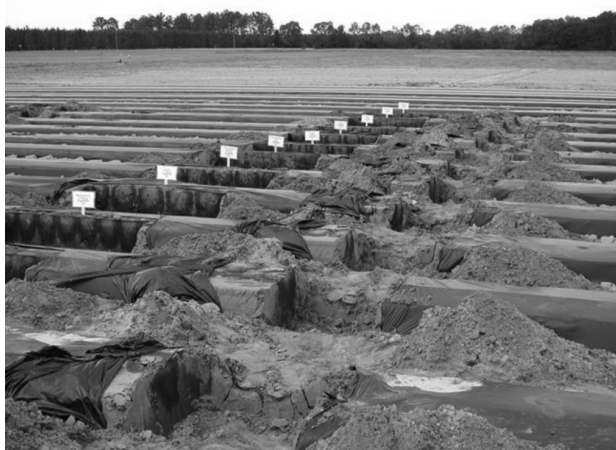
FIGURE 5 Overview of a dye test conducted on a Blanton-Foxworth-Alpin complex (formerly Lakeland fine sand) at the UF/IFAS Suwanee Valley Agricultural Extension Center, Live Oak, FL, showing longitudinal (left) and transverse (right) sections of the bed (Photo credit: Eric Simonne, University of Florida).
