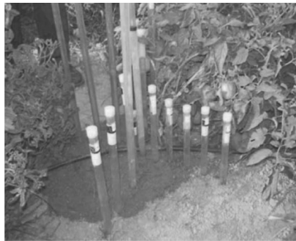
FIGURE 4.2 Measurement of wetted front advance: Visual and tensiometric (sensors).
