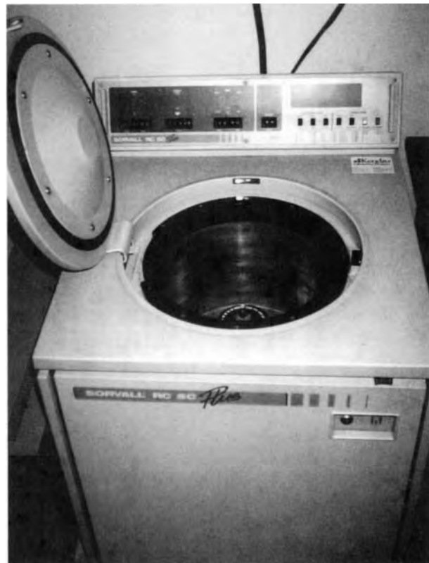
Fig. C.20: A cooling, high-speed centrifuge.
