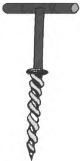
Fig.S.13: Soil auger, a tool used in soil sampling.
