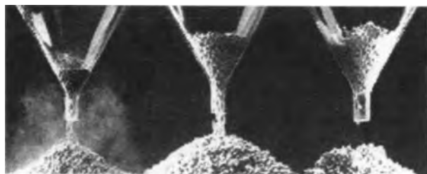
Fig. C.1: Flowability of a fertilizer in a free particulate state and its non-flowability, when caking occurs.
