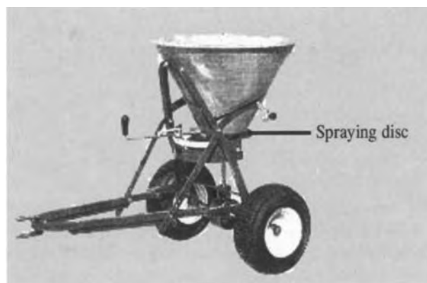
Fig.F.14: A broadcast spreader with a spinning disk. (Source: www.daken.com.au/images/fertspred/rond_spt160_man.jpg . With permission from Dr. Verther Rondini of Rondini Company, Italy.)
