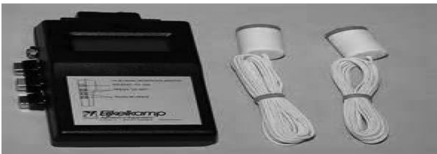
FIGURE 3.9 Gypsum blocks with an instrument to measure electrical conductivity of soil moisture.
