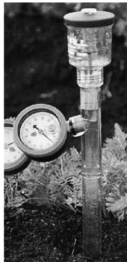
FIGURE 5.9 Tensiometer based irrigation scheduling.
