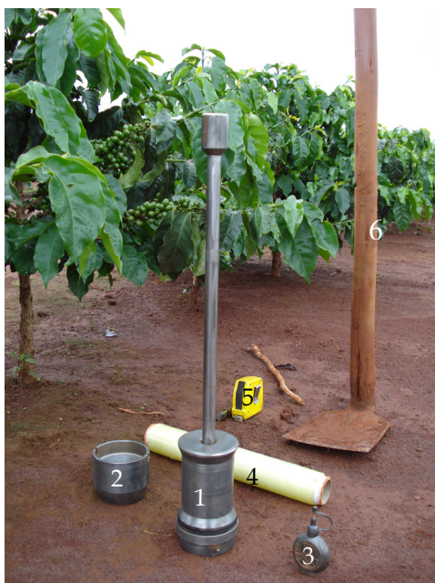
Photo 2. Uhland undisturbed soil sampler components. 1 - driving assembly; 2 - aluminum cylinder room ; 3- graphite lubricant; 4 - plastic film to cover soil sample; 5 - measuring tape; 6 - mattock for digging soil sampling pit.
