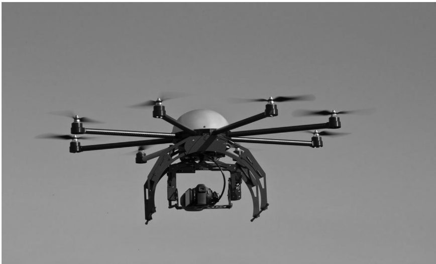
PLATE 3.13 A Multi rotor (Octocopter) Drone in the Air, showing the scanning camera/sensor
