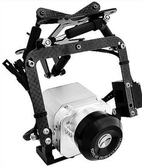
PLATE 3.19 A Camera for Thermal Imagery of crops with fixtures that fit the agricultural drone (Note: Cameras capable of imagery at infra-red band width are used to assess crop water status. Most drones carry a complement of cameras that includes thermal imaging. Source: commercial websites.).
