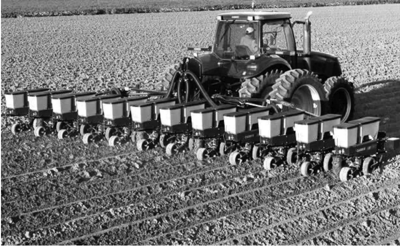
PLATE 4.9 Variable-Rate Planters (Source: Dr. Daniel Danford, CEO, CaseIH Inc., Oakes Rd., Sturtevant, Wisconsin, USA).
