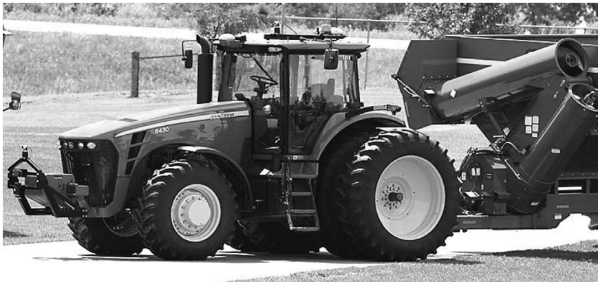
PLATE 2.24 A close up view of Kinze's Autonomous Grain Carting Vehicle (Source: Kinze Manufacturers Inc., Williamsburg, Iowa, USA; Note: This robotic vehicle is controlled by wireless or GPS guidance system. It shuttles all along the fields, from one combine harvester to another, from combine to transport vehicle, etc. The Robotic grain cart can be programed and controlled using computers located in a cabin nearby or by a technician situated on farm bund using a computer tablet. The grain cart could be controlled using touch screen system on a tablet. The Autonomous Grain Cart (Driverless!) along with Robotic Combine harvesters are excellent examples of the forecasted 'Push Button Agriculture.').
