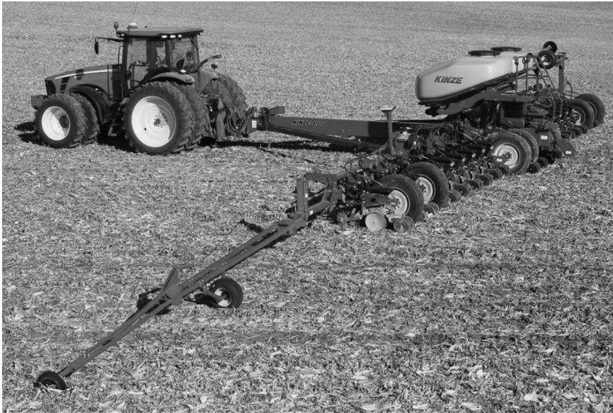
PLATE 2.10 Robotic Seed Planters in use in a Farm in North America (Source: Kinze Manufacturers Inc., Iowa, USA; Note: An autonomous tractor with GPS guidance and variable seed rate facility operating on Mollisols (Chernozems) of USA. Steer less tractors are becoming more common in the agrarian zones of North America and Europe).
