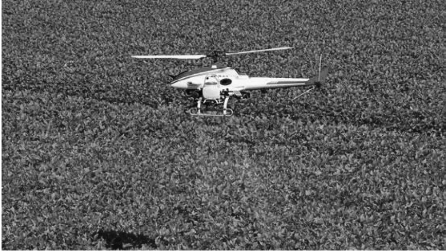
PLATE 3.9 Yamaha RMAX Drone (Note: RMAX is a popular drone among Japanese Agriculturists. RMAX flying at low altitude over a soybean crop. It is spraying pesticide on the crop. Source: Yamaha Motor Co, Australia, http://rmax.yamaha-motor.com.au/agricultural-use ; Barnard Microsystems Inc., http://global.yamaha-motor.com/about/business/sky/ ).
