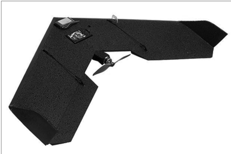
PLATE 3.3 Swinglet CAM (Source: Dr. Mathew Wade, Sensefly, Cheseaux-Lausanne, Switzerland; Note: Swinglet CAM is a small Fixed-wing Drone useful for Mapping Natural resources and Agricultural crop scouting. The entire drone and accessories fit into a small suitcase and are easily portable to any location).
