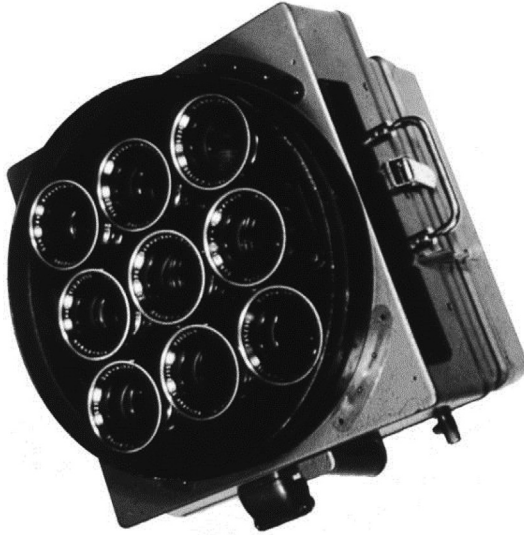
PLATE 3.18 A Multispectral Camera that can be fitted to drones (Note: There are several types and models of multispectral cameras used on drones; Source: Commercial advertisements in web sites.).
