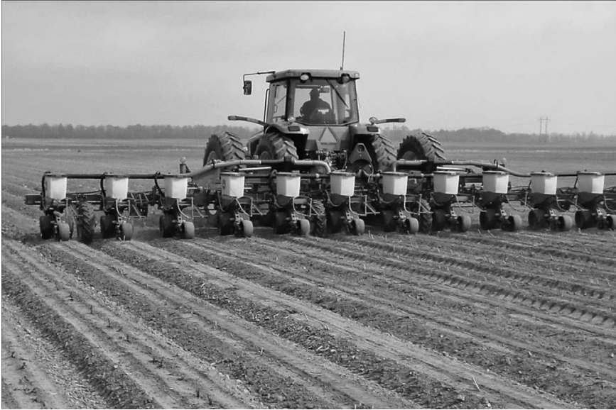
PLATE 2.7 Corn Seed Planter-A Semi-autonomous Robot used widely all over the Agricultural zones of the world (Source: Mr. David Nelson, Nelson Farms, Iowa, USA; Note: Tractor speed and settings on seed bins decide the rate of seeding. Seeding could be made accurate if GPS guided and variable-rate seed planters are used).
