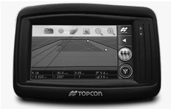
PLATE 2.8 Left: Touch Screen GPS Guidance console-example; Right: A Robotic Steering Control System-example (Source: Mr. David Nelson, Nelson Farms, Iowa, USA; Note: The touch screen guidance allows farmer to verify the areas already planted with seed. Planter could be selectively moved to areas that need planting. It can be used to adjust planting speed, seed density, replanting spots that were devoid of seeds, etc. The GPS guidance equipment could also be used to regulate variable-rate applicators regarding fertilizer/irrigation and water supply to entire field).
