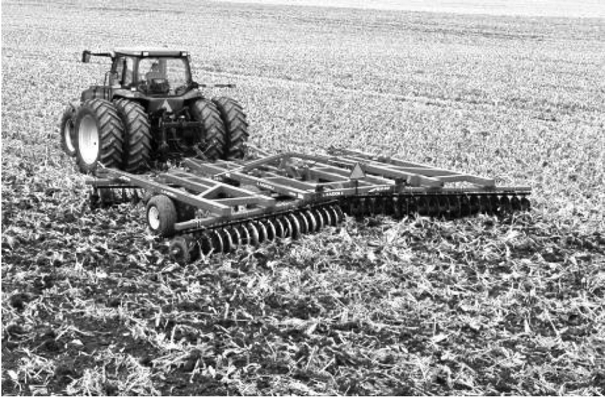
PLATE 2.3 A semi-autonomous tractor (not driverless) plowing (disking) wheat field in Kansas, USA (Source: Mrs. Paula Landoll-Smith, Landoll Corporation, Marysville, Kansas, USA).
