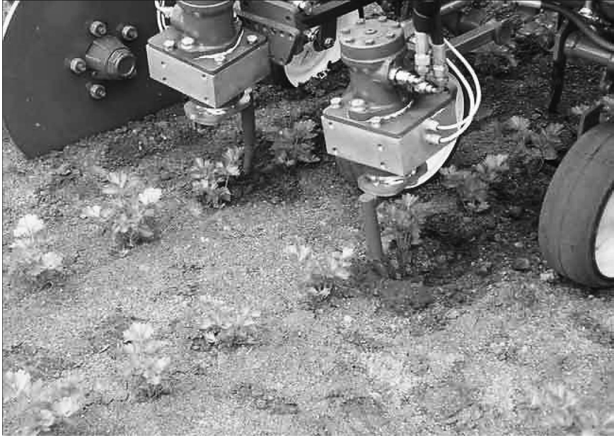
PLATE 2.19 Robotic Weeding Machine (Source: Dr. Philip Garford, Garford Farm Machinery, Peterborough, England; Note: These Semi-automatic robotic machines are programmed to apply herbicides at specific spots).
