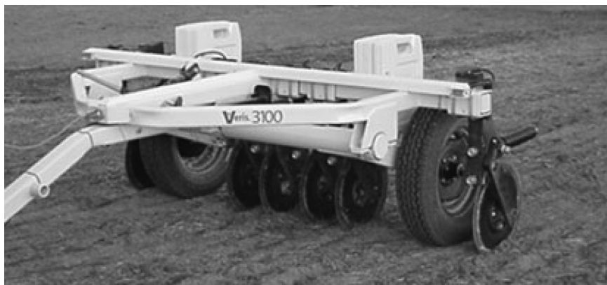
PLATE 4.8 A Soil Electrical Conductivity Sensor (Source: Mr. Eric Lund, Veris Technologies Inc., Salina, Kansas, USA http://www.veristech.com/products/soilec.aspx (August 1 st , 2011); Note: Soil EC Mapper detects changes in soil EC and maps it ‘on-the-go’ using soil surface contact technique. Soil EC is supposedly indicative of several soil traits such as texture, SOM, salinity and soil moisture holding capacity. Indirectly it measures soil productivity).
