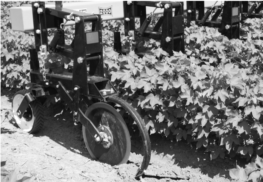
PLATE 2.6 The Landoll 2000 Series Row Crop cultivator for earthing up, aeration and weeding (Source: Mrs. Paula Landoll-Smith, Landoll Corporation, Marysville, Kansas, USA; Note: Row crop cultivators are excellent in disturbing the inter-row soil mildly. They rip and stir the surface layer of soil. Cultivators are used when the intension is to induce oxygenation of soil, turn the soil and induce rooting of crop. They are also used just prior to placing fertilizers in a band).
