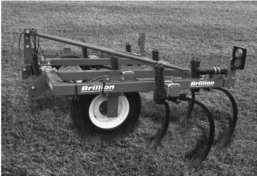
PLATE 2.2 Chisel Plow (Source: Mrs. Paula Landoll-Smith, Landoll Corporation, Marysville, Kansas, USA; Note: Chisel plows are part of primary tillage systems. These are pulled by semi-autonomous driver operated tractor. They are useful when land is rugged, with excessive residue and stones. Chisel plows are used when practicing ‘Conservation tillage.’ It is still a very popular plow in the Great Plains of North America).
