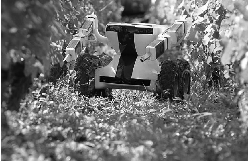
PLATE 2.29 Wall-ye, the grape vine robot searching for fruit bunches (Source: Dr. Christophe Millot- inventor and Dr. Guy Julian- Manufacturer. http://www.kare11.com/video/1860715174001/1/wall-Ye-Wine-Robot-takes-bow-in-Burgandy (June, 23 rd , 2014)).
