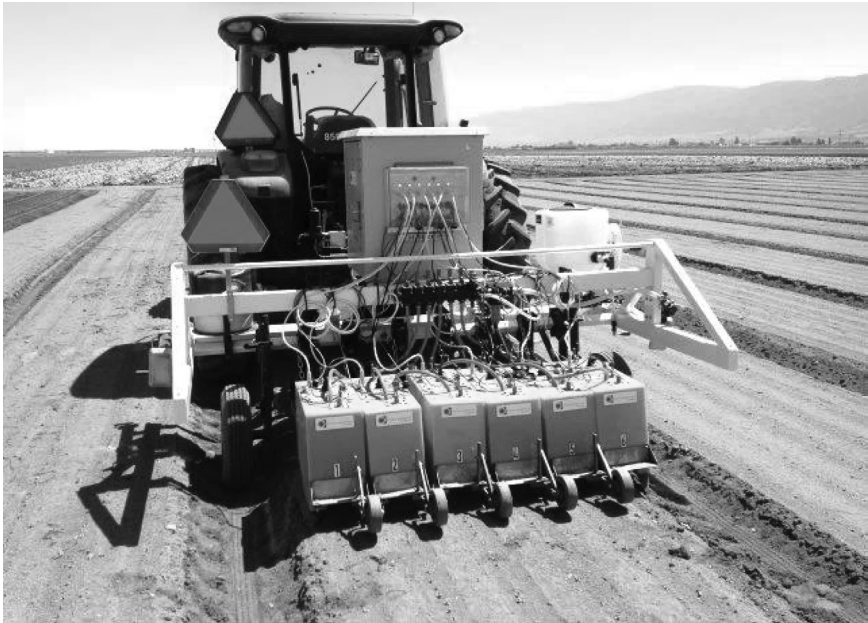
PLATE 2.26 Lettuce Crop Thinner (Source: Dr. Tony Koselka, Vision Robotics, San Diego, CA, USA; Note: During lettuce production, appropriate spacing and thinning of plants is essential to maintain a good crop. The quality of foliage and value of vegetable is dependent on intra-row spacing. The above robot is endowed with sensors that allow the robot to identify less developed plant and selectively thin them).
