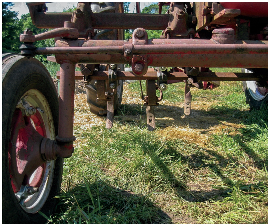
FIGURE 5.4. Cultivator shovels for furrowing mounted on the tractor toolbar allow for fast work where long furrows are needed.
