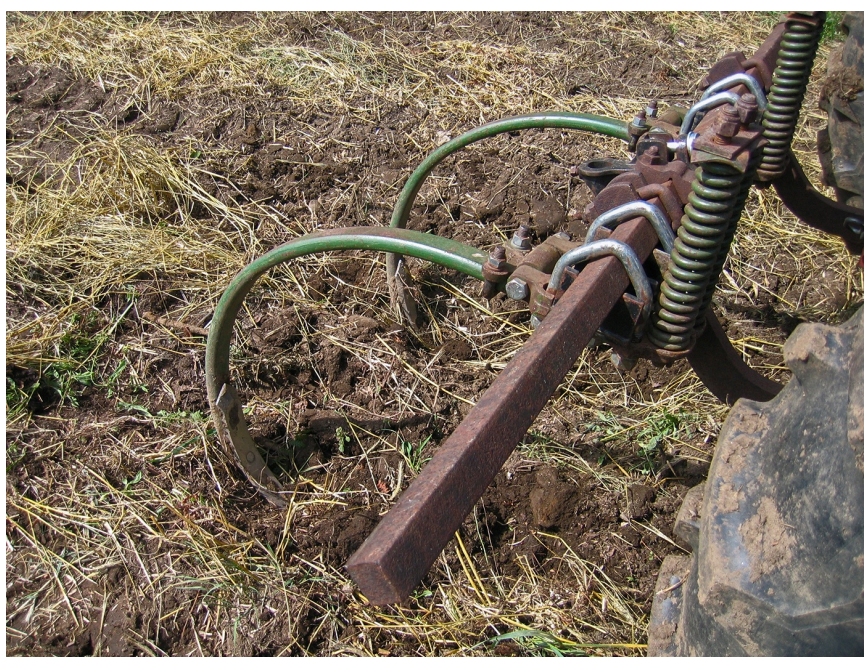
FIGURE 3.3. A chisel plow can cut deep but produce minimal soil disturbance, even in a high-residue environment.
