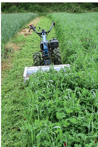
FIGURE 4.2. We use the BCS flail mower to cut down dense cover crops before solarizing.
