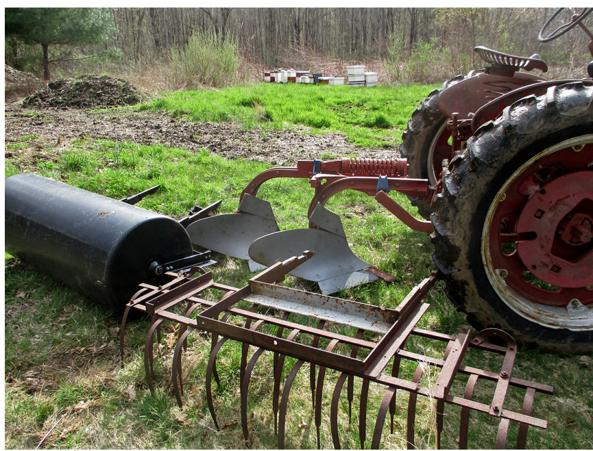
FIGURE 3.2. Our tractor-mounted tillage tools include a moldboard plow, a tined rod weeder, and a water-filled drum roller. We use these when converting new growing areas to no-till.
