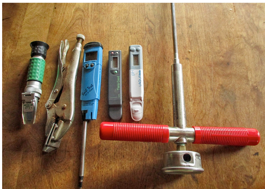
FIGURE 8.1. On-farm plant and soil assessment tools include a refractometer and adjusted vise grip for extracting and assessing plant sap, three types of electrical conductivity and pH meters for both soil and sap analysis, and a penetrometer for testing soil compaction.
