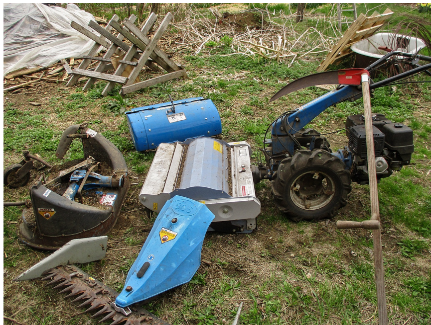
FIGURE 4.1. We mow using this BCS two-wheeled tractor and various attachments: a flail mower (mounted on the BCS), the
