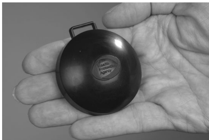
Figure 5.2 Passive Radon Metre. Adapted with kind permission from Report HPA-RRP-001 'Ionising Radiation Exposure of the UK Population: 2005 Review' by S J Watson et al (2005), © Health Protection Agency.
