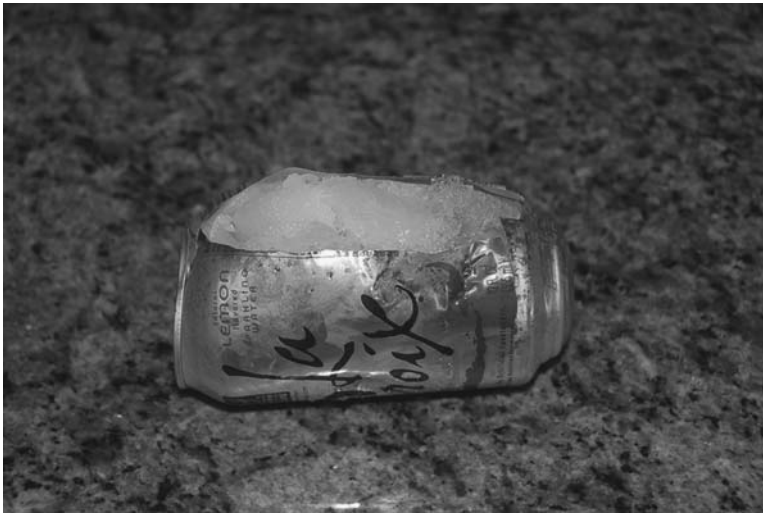
Figure A19.4 This can of water was left outside on a cold night. Notice that it has burst due to the expansion of the ice inside.
