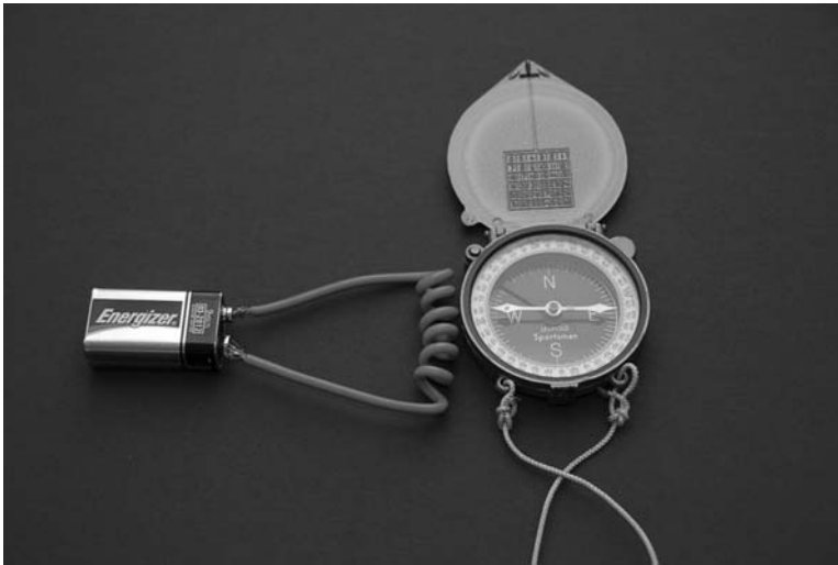
Figure 1.1 This arrangement of a battery, wire, and compass can be used to demonstrate the interaction of magnetism and electricity.
