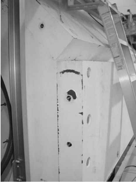
Figure 1.2 These large iron blocks are positioned within the housing of a superconducting magnet to make the magnetic field more compact. This allows the MR scanner to be placed in a room that may have formerly housed a CT scanner because the fringe field is now smaller.
