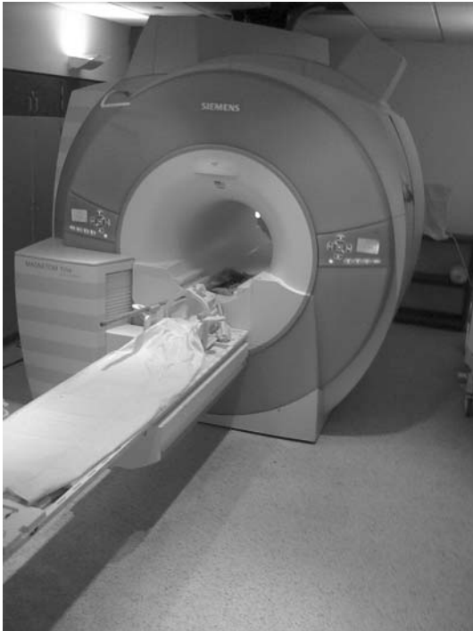
Figure 1.26 This mop, stuck inside the bore, was brought too close to the magnet and it proved to be difficult to pull it out. In the radiology department, it is essential to remember that both X-ray radiation and strong magnetic fields are invisible but ever-present risks to you, your colleagues, and your patients. Unlike similar-sized X-ray devices in the department like CT scanners and angiography units, the strong magnetic field of an MR scanner is never turned off.
