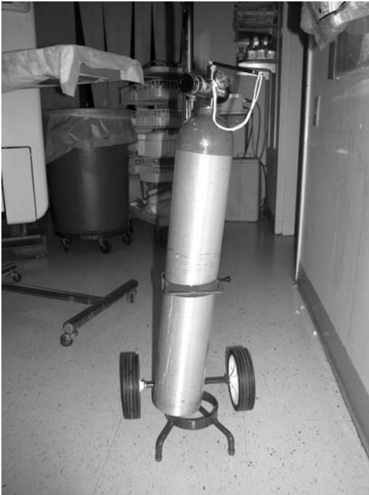
Figure 1.29 While this is a nonferrous (aluminum) oxygen tank and can therefore enter the MR scanner room, be aware that it may be sitting in a ferrous cart.
