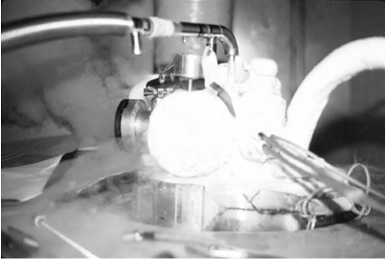
Figure 1.5 Frost forms on the cold head at the top of the MR scanner where moisture in the air freezes as it meets the extreme cold due to the liquid helium within. This device provides access to the magnet for the helium refills.
