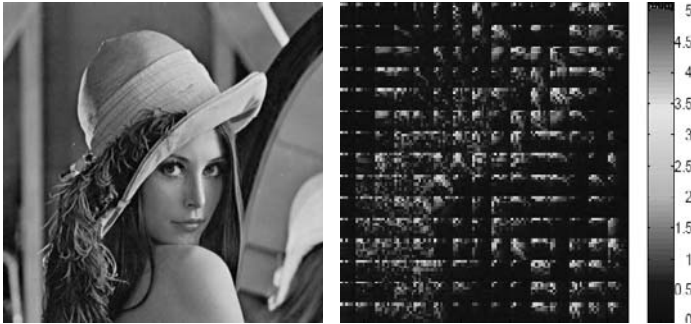
Figure 2.4. Local spectral DCT domains of the image Lena (with absolute values of the coefficients shown in false color): we can see the real difference between the local spectral signatures
