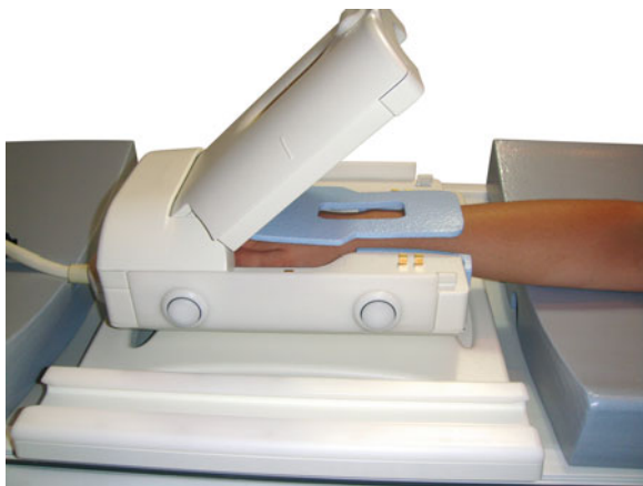
Figure 8.19 A sample head first and prone patient positioning for a dedicated, multichannel wrist coil is shown. Please note that the coil stands horizontal here and wrist is placed in the coil palm on the table.
