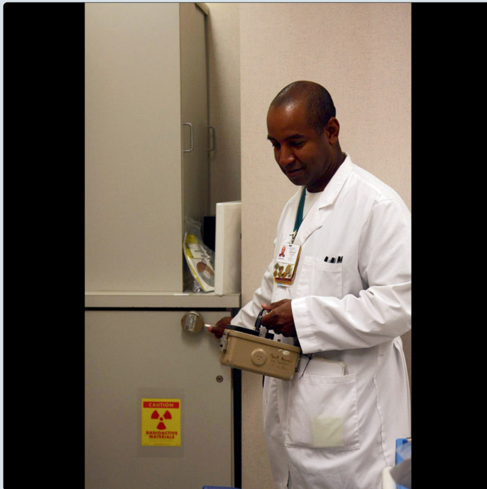
Technologist is shown performing a survey in a restricted area using a Geiger-Müller survey instrument. He is assessing the radiation level in the room and storage device as compared to background radiation levels. Occupational doses are affected by background radiation in the department.
