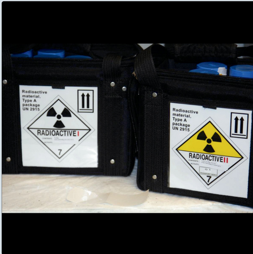
White I and yellow II packaging shown. The yellow II has a transportation index, which is the radiation exposure at 1 m. The shipping and receiving of packages is regulated by the Department of Transportation.
