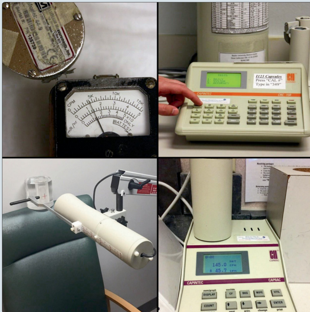
Gas-filled and scintillation detectors are shown: Geiger Müller (GM) gas-filled detector (top left) reads out in units of mR/hr; dose calibrator gas-filled detector (top right) typically reads out in mCi or MBq; thyroid uptake probe scintillation detector (bottom left) reads out in disintegration per minute (dpm); and well counter scintillation detector (bottom right) reads out in counts per minute (cpm) or disintegrations per minute (dpm) when radionuclide efficiency is taken into account.
