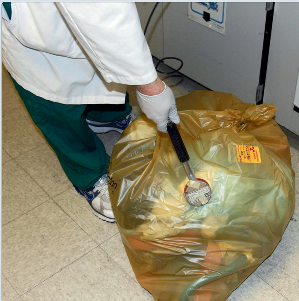
Technologist uses a Geiger-Müller detector to survey decay-in-storage material. Once the activity equals background levels, the radioactive labels are destroyed and the trash can be placed with regular trash.
