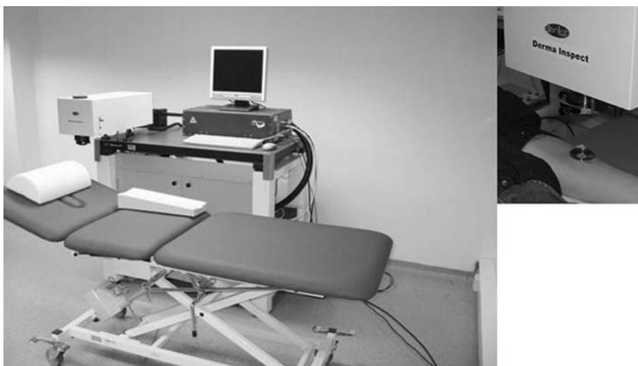
FIGURE 4 Photograph of the multiphoton imaging tool DermaInspect 110 ® for four-dimensional autofluorescence and second harmonic generation imaging with intracellular spatial resolution (around 1 \mu\text{m} ) and 250 psec temporal resolution.
