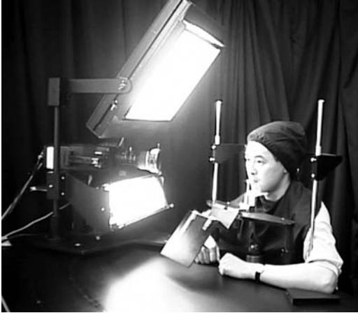
FIGURE 1 Facial imaging system composed of a light source, dimmer switch, 3-CCD video camera, computer, and positioning device for accurate alignment of the subject's face.
