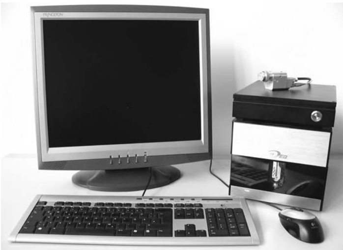
FIGURE 6 Prototype of a spectral radar no-motion optical coherence tomography (OCT) built by the medical laser center Lübeck GmbH/Thorlabs HL AG, Germany. The compact device has a small handheld applicator connected by optical fibers.
