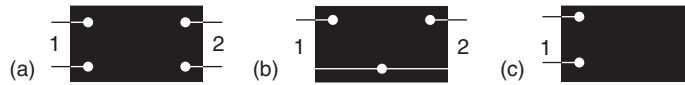
Figure 7.1 Black boxes. The two boxes (a) and (b) allow for transfer parameters from one port to the other. Box (c) is a one-port, two-terminal box with only driving point parameters possible.
