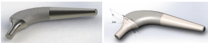
Fig. 12 Biomedical implants with dimensions produced by investment casting
