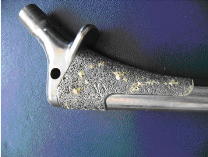
Fig. 9 Example of currently used surface finishing technique for hip prostheses stems
