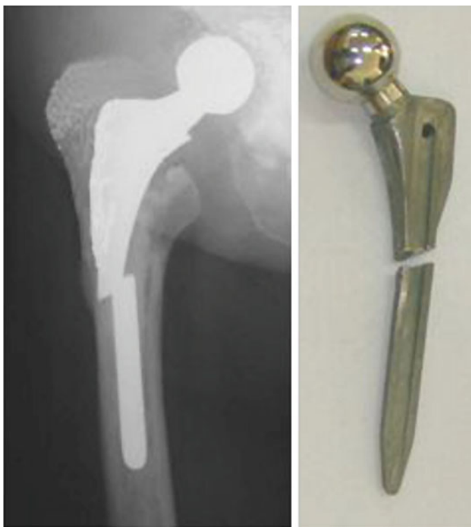
(a) Radiographs of the broken hip (b) Broken hip implant after surgery
