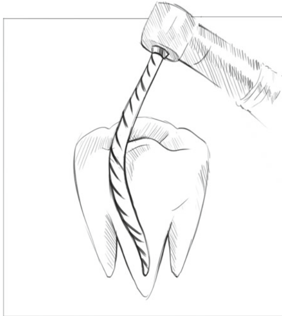
Fig. 16 Orthodontic applications of SMA: scheme of NiTi drill used for root canal surgery (Lagoudas 2010)
