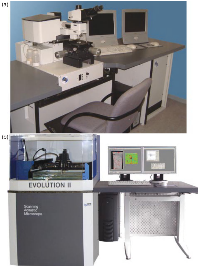
Figure 12.3. Two acoustic microscopes that are distributed by PVA Tepla (Westhausen, Germany). (a) High resolution instrument “Evolution PII” ( f \leq 2 GHz) with integrated light microscope. In this image, the head with the acoustic scanner is moved toward the left. (b) Instrument of the Evolution-series (Evolution II) in the frequency range between 3 and 400 MHz with large motorized scan width for samples up to 520 \text{ mm} \times 380 \text{ mm} \times 45 \text{ mm} (w/l/h) and water tank for the specimen. (Images courtesy of PVA Tepla, Westhausen, Germany).
