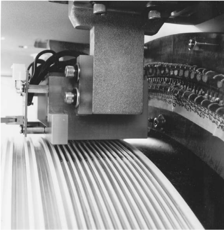
FIGURE 9.6 Photograph of the slip rings used to pass power and control signals to the rotating gantry. (Courtesy of Picker International, Inc.)
