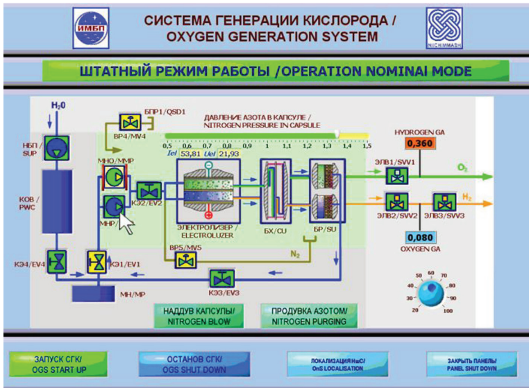
Fig. 11. Front panel of the 'OGS' virtual simulator subroutine in 'OPERATION NOMINAL MODE' (НБП/SUP=supply unit pump; КОВ/PWC=pre-purification water container; КЭ1/EV1=electromagnetic valve; МНО/ММР and МНР/МРР=main micro-pump and reserve micro-pump; БХ/СУ=cooling unit; БР/СУ=separator unit; GA=gas analyzer).
