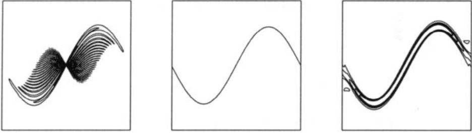
Fig. 4.2.3: Inner interference terms in the time-frequency analysis of a chirp signal. In the WVD case (left), cross-terms appear midway between any two points belonging to the instantaneous frequency trajectory (middle). As for the “outer” interference terms of Figure 4.2.2, these “inner” interference terms can be reduced by using a smoothed pseudo-WVD (right).
