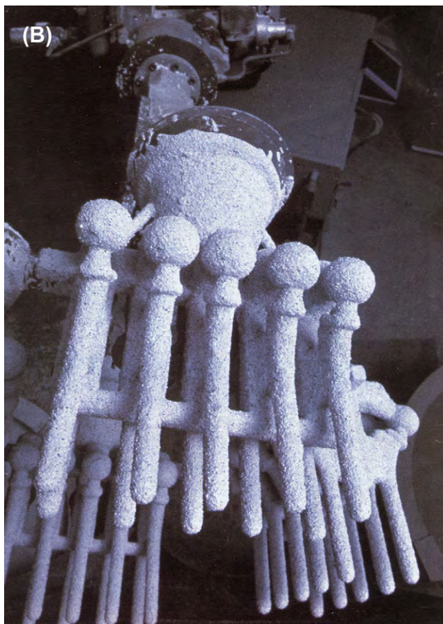
FIGURE 1.2.3.1 (B) Image of one step during the investment casting ("lost wax") process of manufacturing hip stems; a rack of hip stems can be seen attached to a system of sprues through which molten metal can flow. At this point, ceramic investment material composes the mold into which the molten metal will flow and solidify during casting, thereby replicating the intended shape of a hip stem.
