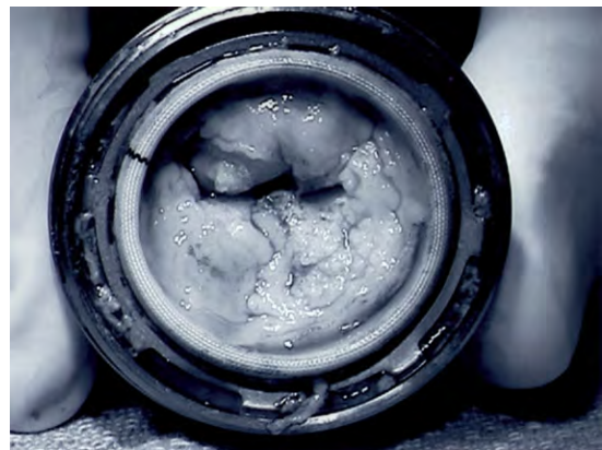
FIGURE D.8 Candida albicans vegetations partially obstructing the inflow valve of a Novacor VAD patient at the time of valve replacement. (Kindly provided by R. L. Kormos, M.D, Director, and S. Winowich of the University of Pittsburgh Medical Center Mechanical Circulatory Support Program.).
