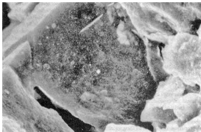
FIGURE II.4.2.20 Smooth crack wall indicative of brittle fracture caused by metal ion-induced oxidation (×830).
