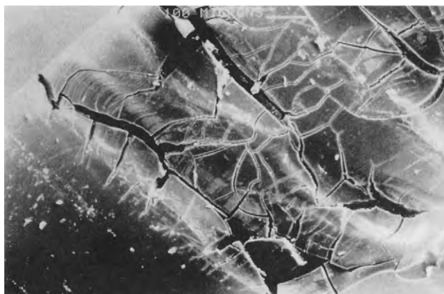
FIGURE II.4.2.21 Crack pattern on inner lumen of polyether urethane lead insulation tracking coil indicative of metal ion-induced oxidation (×100).
