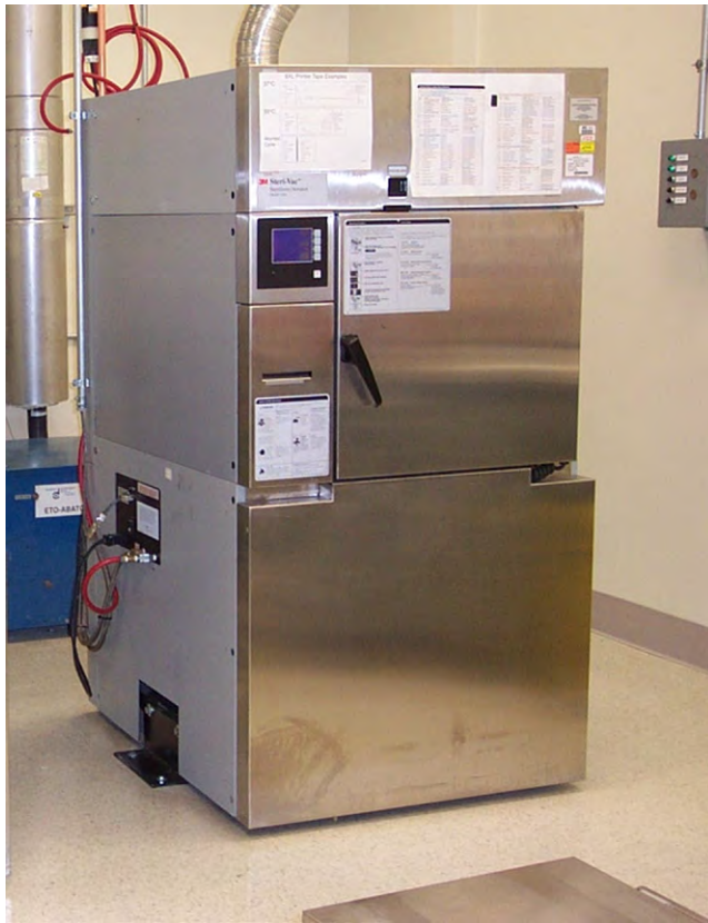
FIGURE III.1.2.6 Low volume ethylene oxide R&D sterilization chamber (Courtesy of Getinge Inc.).
