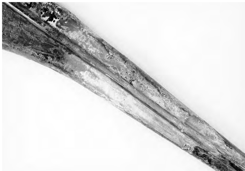
FIGURE II.4.4.5 Extensive corrosion on the titanium stem of a modular hip prosthesis.
