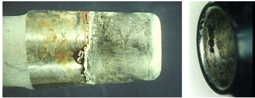
FIGURE II.5.6.15 Modular junction taper connection of a total hip arthroplasty showing corrosion of the taper connections. Macrograph of deposits of \text{CrPO}_4 corrosion particles on the rim of a modular cobalt–chrome femoral head.
