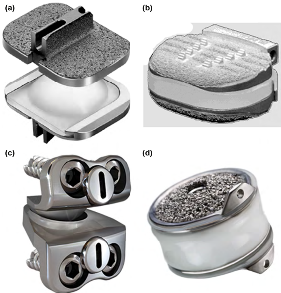
FIGURE II.5.6.6 Cervical IDRs (Intervertebral Disc Replacement): There are a number of cervical total disc replacements in use which employ the three primary types of disc joint articulation. 1. Metal-on-Polymer Articulation: (a) The PRODISC-C® (Synthes, Inc.); and (b) PCM® (Cervitech); use Co-alloy endplates that articulate on a polymeric (UHMWPE) core that is mechanically fixed to one of the endplates and articulates in a ball-and-socket type manner. 2. Metal-on-Metal Articulation: (c) The PRESTIGE® Disc (Medtronic) has metal-on-metal articulation where the end plates are constructed of stainless steel. 3. Elastic Core Articulation: (d) The Bryan® Cervical Disc System (Medtronic) is axially symmetric and incorporates cobalt-chrome alloy clamshell-shaped endplates, which flex upon a loadbearing polymeric (polyurethane-based) nucleus core. A novel feature in the design of this component is the polyurethane flexible membrane that surrounds the entire articulation and forms a sealed space containing a saline lubricant to reduce friction and prevent migration of any wear and corrosion debris. (Pictures provided courtesy of DePuy Spine, Inc., Medtronic, Spine Solutions, Inc., and BioEngineering Solutions, Inc.)
