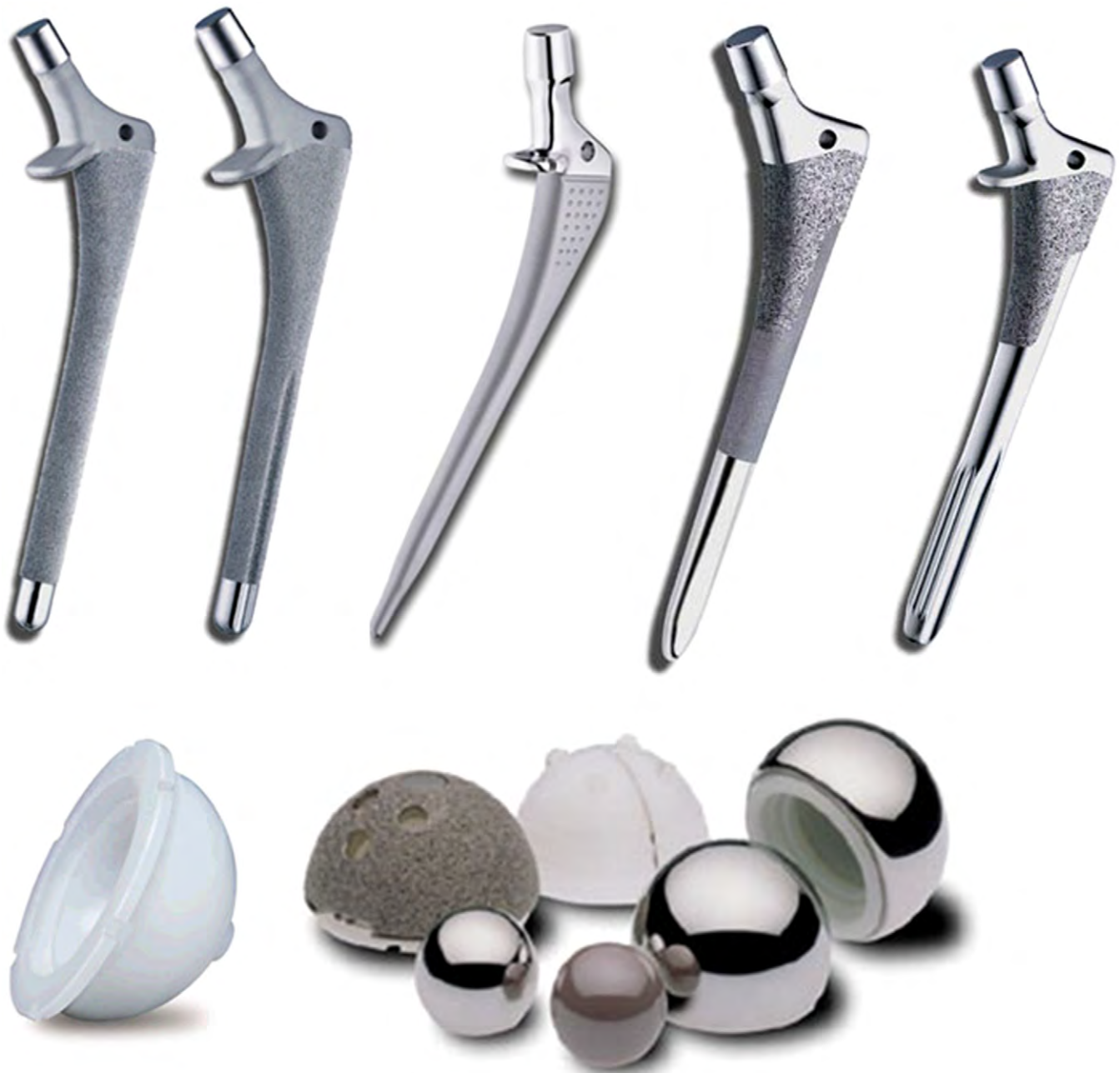
FIGURE II.5.6.8 Examples of typical current total hip arthroplasty (THA) components available from a single manufacturer: titanium alloy stem, with a cobalt-base alloy (ASTM F-75) modular head bearing on an ultra-high molecular weight polyethylene (UHMWPE) liner within a titanium alloy cup. Also shown are a ceramic head and three acetabular sockets with various surfaces for both cemented and cementless fixation. From left to right the stems are all components of the VerSys® Hip System (Zimmer, Inc, Warsaw, IN, USA), and from left to right are designated Beaded Fullcoat, Beaded Fullcoat with distal flutes, Cemented, Fiber Metal Taper, and Fiber Metal Midcoat. (Photographs courtesy of Zimmer, Inc.)
