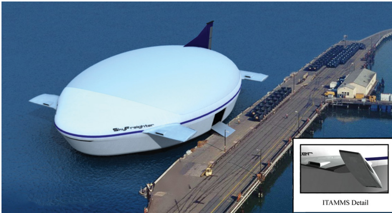
FIGURE 23.15 The SkyFreighter, a very large capacity hybrid air vehicle, capable of landing and takeoff from the sea or land. Source: Millennium Airship, Inc. Reproduced with permission.
