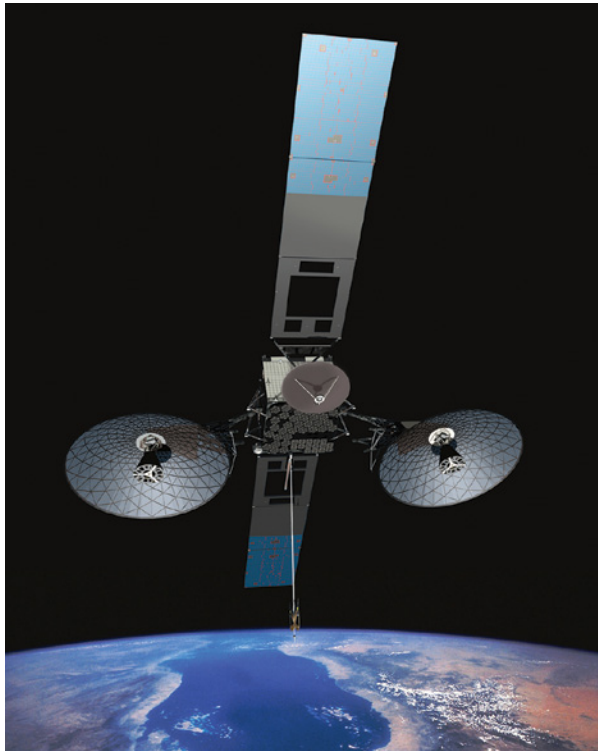
FIGURE 16.16 Picture of TDRS (Gen 2) deployed by the space shuttle, but prior to orbital transfer to high earth orbit. Source: NASA.
