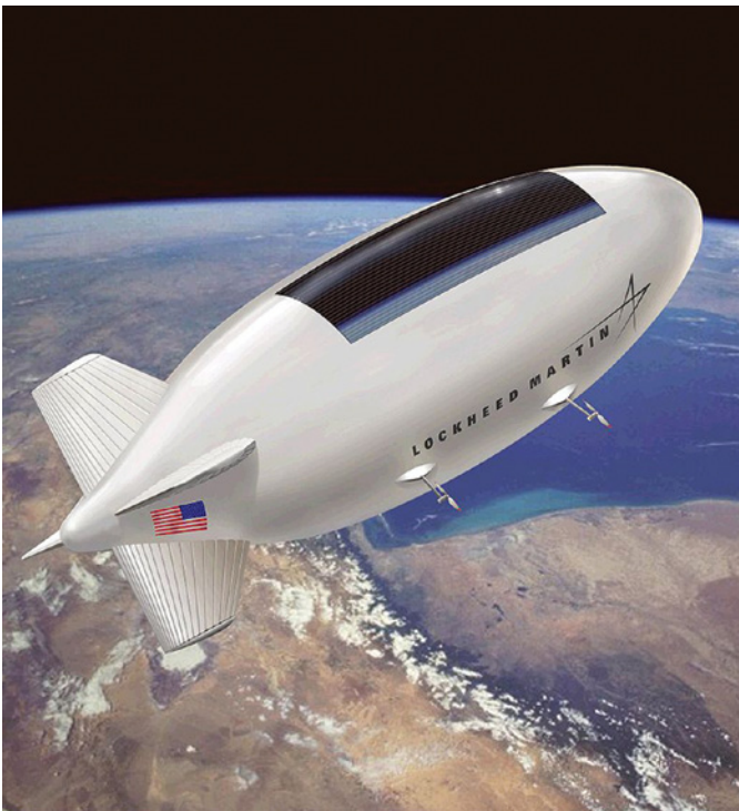
FIGURE 23.14 The solar-powered High-Altitude Long-Endurance Demonstrator (HALE-D). Source: U.S. Air Force.
