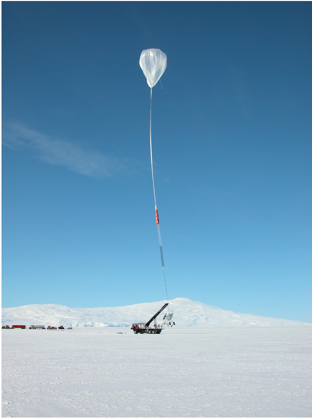
FIGURE 23.11 The mobile crane moves the payload directly beneath the balloon. Source: NASA/Columbia National Balloon Facility.
