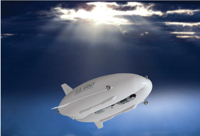
FIGURE 23.13 The High Altitude Airship (HAA) developed for the U.S. Army Space and Missile Defense Command. Source: U.S. Army.
