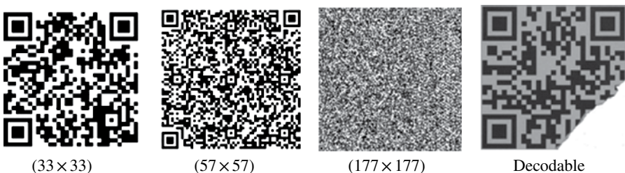
FIGURE 3.5 The 2D QR code that has become a popular product and service identification code. From left to right: Version 4, Version 10, Version 40, and a damaged QR code from which all information can be recovered. Credit: Compilation from Wikipedia public domain images.
