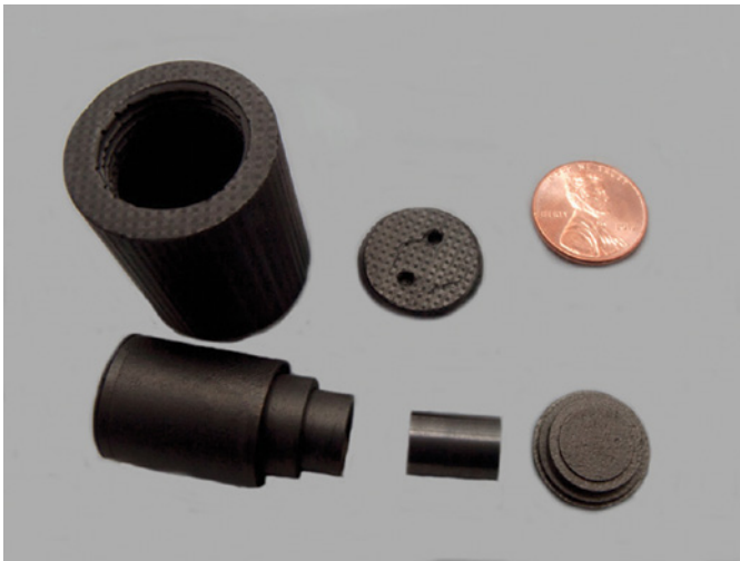
FIGURE 16.15 The components of a single lightweight radioisotope heater used to provide supplemental heat sources for deep-space satellites. The penny provides a size comparison.
