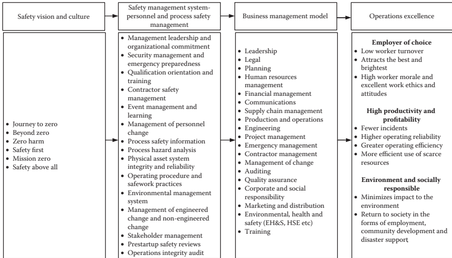
FIGURE 7.3 Safety culture and its influence on operational excellence (OE). (Adapted from Suncor Energy Inc., copyright of Suncor Energy Inc., approval from Suncor is required to reproduce this work.)
