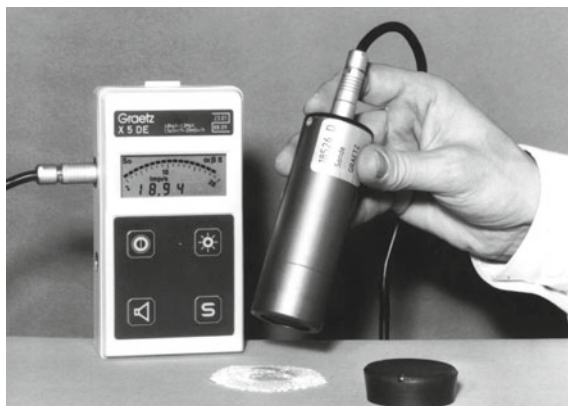
Fig. A.3 Taking a measurement of activity with a Geiger-Müller counter. (Tube 18526D and counter X5DE, from GRAETZ, Altena, Germany)
