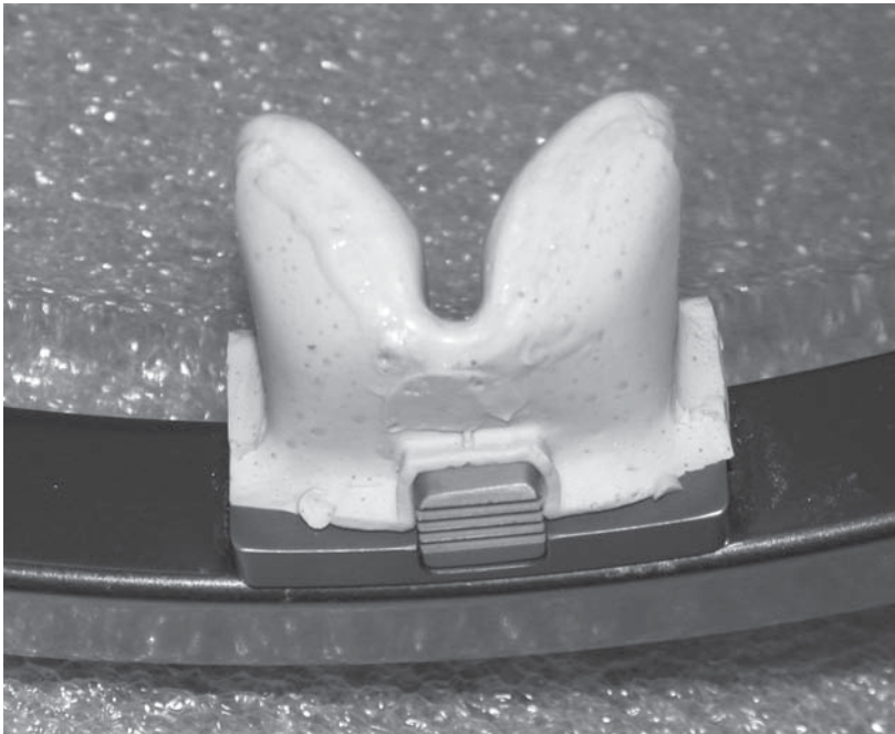
24. The Apollo-version Valsalva device, used to help astronauts equalize the pressure in their ears, is clearly visible attached to the helmet base ring.
