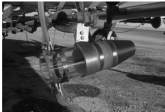
Figures 26.4 Devices are under development for the aerial application of Trichogramma (as parasitized host eggs) in orchards: (a) release device on wing, (b) plane, and (c) close up of release device. Photographs courtesy of Nick Mills.
