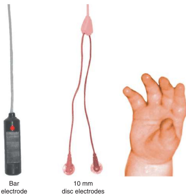
FIGURE 38-2 Pediatric electrodiagnostic studies and recording electrode size. The standard bar electrode ( left ) and 10 mm disc electrodes ( middle ) are compared to the size of an infant's hand ( right ). Smaller electrodes may be needed in infants and young children because their limbs and muscles are so small. Standard 10 mm disc electrodes often will suffice for most age groups, including infants. In newborns, however, smaller electrodes are needed. Other standard electrodes, like the bar electrode, are too large for a newborn or infant's hand.
