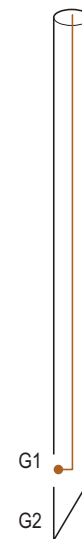
FIGURE 34-3 Single-fiber electromyography needle. The active electrode (G1) is located in a port along the posterior shaft of the needle, with a smaller leading surface area than a conventional concentric needle electrode. The reference electrode (G2) is the needle shaft.
