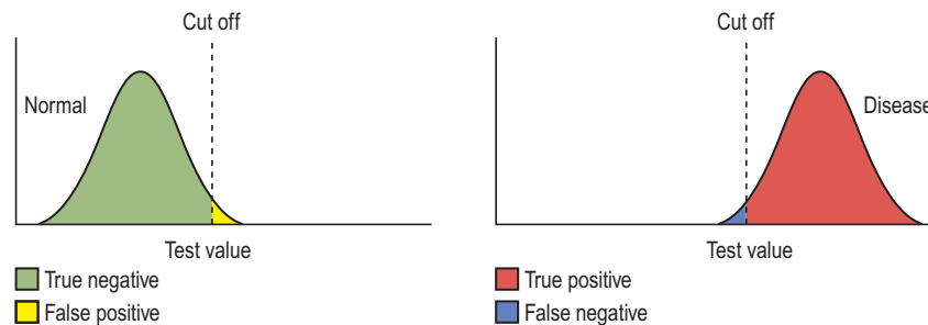
FIGURE 9–2 Cutoff values and false results. Left: When a test is applied to a population of normal patients, the test will correctly identify all patients who are below the cutoff value as normal (true negative [green in the figure]); however, it will misidentify a small number of normal patients who are above the cutoff value as abnormal (false positive [dark blue in the figure]). Right: When a test is applied to a disease population, the test will correctly identify all abnormal patients who exceed the cutoff value (true positive [red in the figure]); however, it will misidentify a small number of abnormal patients who are below the cutoff value as normal (false negative [dark blue in the figure]).
