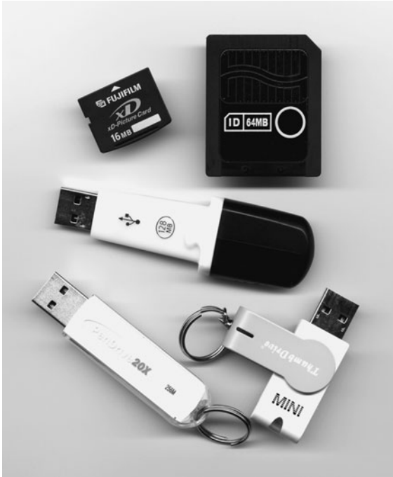
Figure 11.6 A selection of removable storage devices using flash memory. Their capacity ranges from 16 MB (top left) to 1 GB (bottom right). The bottom three devices use USB connection.
