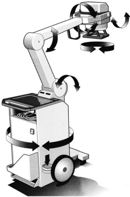
Figure 9.9 A small mobile X-ray unit showing the considerable maneuverability of the body and arm. The generator is integrated within the X-ray tube housing. The body contains the battery and charger unit. (Courtesy Siemens Inc.)
