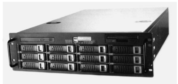
Figure 11.10 A commercial server which has a bank of twelve hard disks giving a total of 4.8 TB.
