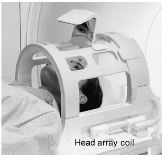
Figure 20.7 Various coil arrays designed for specific anatomical regions. Their application significantly increases the image signal to noise ratio (courtesy of Siemens Medical Systems).
