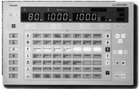
Figure 9.8 Top of high frequency generator control unit showing pre-set clinical program list.
