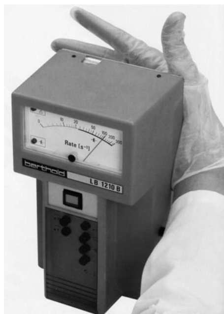
Figure 6.4 Photograph of proportional counter showing large surface area (courtesy of Berthold Inc.).
