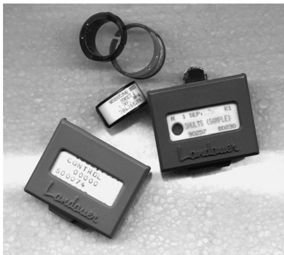
Figure 22.2 A selection of film and thermoluminescence dosimeter radiation monitoring badges. (Courtesy of Landauer Inc.)
