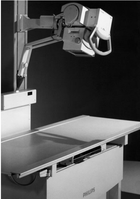
Figure 9.6 A conventional X-ray unit, suitable for general radiography, whose exposure is controlled by feedback from the ion chamber contained in the center of the table top with the Bucky.
