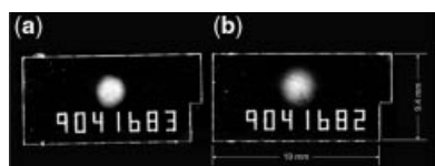
Figure 74 Alpha-particle hits on CR-39 plastic chips after etching for 7 hours in 6 N NaOH at 70^\circ\text{C} . (a) The collimated beam. (b) Alpha-particle beam that has been scattered by a thin gold film.
