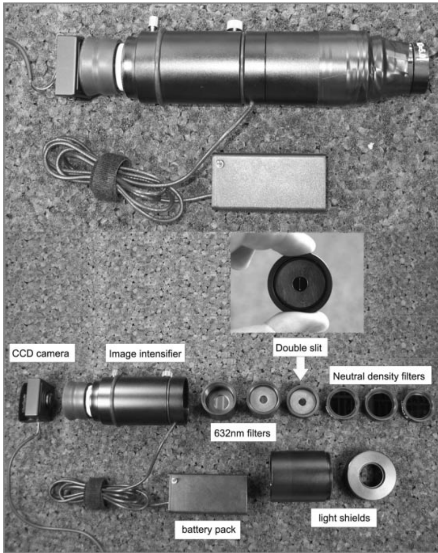
Figure 93 In our single-photon interference setup, a black-and-white CCD camera looks directly at the phosphor screen of a surplus Gen III image-intensifier tube. The interference pattern is projected directly onto the intensifier tube's photocathode.
