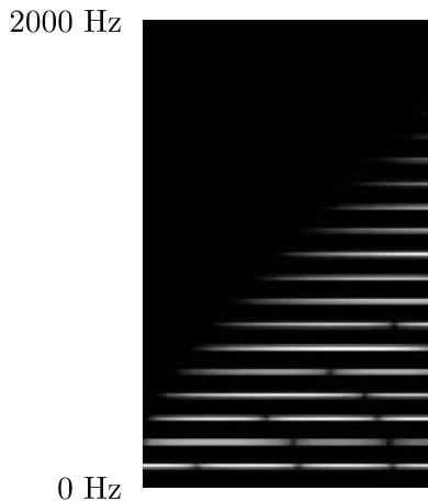
Figure 11.14. A spectrogram for the tone (21) using 0 \leq t \leq 32 sec, T = 1/4000 sec, N = 640 .
