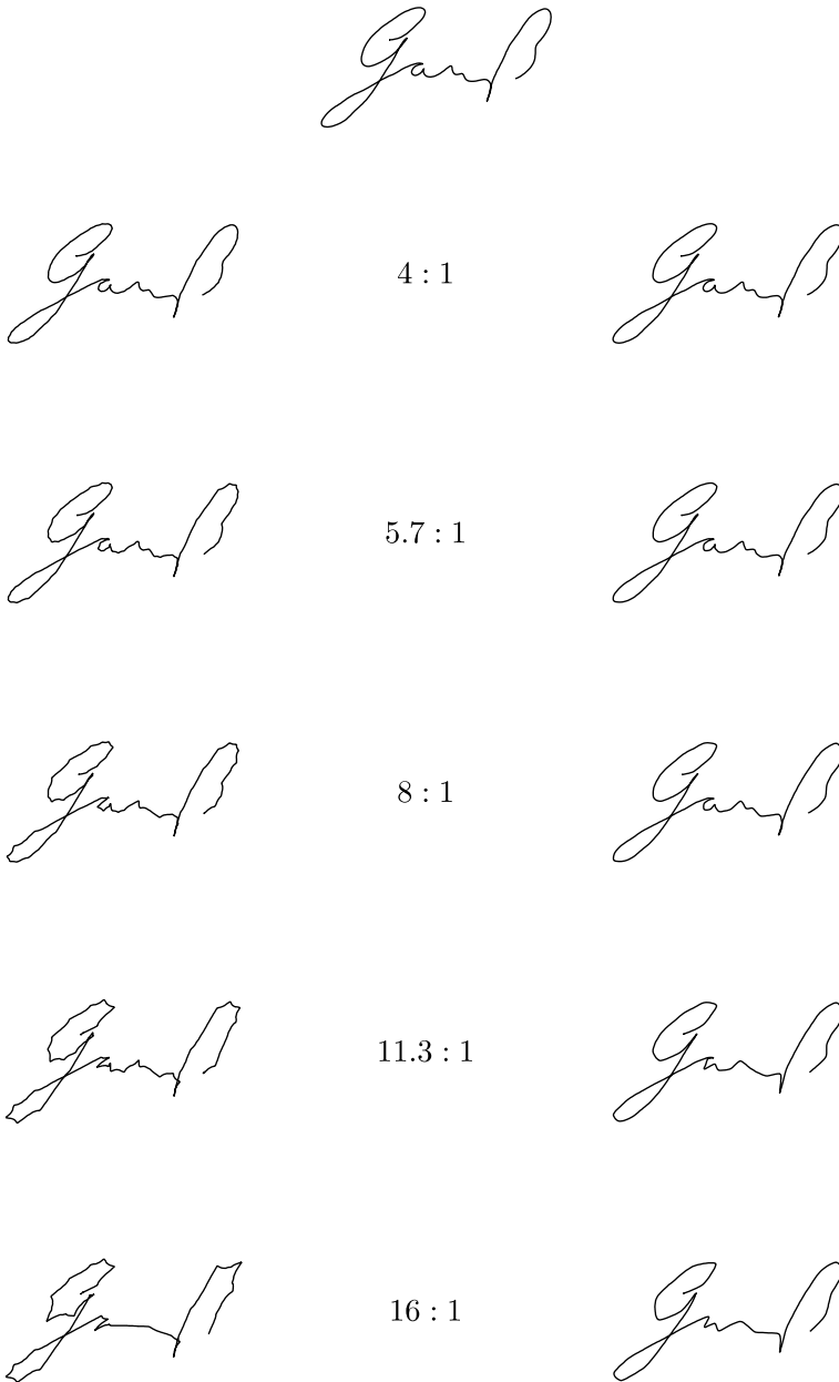
Figure 10.25. A 513-point trace g of a Gauss signature (top) and reconstructions from the 1/4 , 1/\sqrt{32} , 1/8 , 1/\sqrt{128} , 1/16 most significant components of (170) when the filter bank uses the Daubechies coefficients from (39), (148) (left) and the 9/7 FBI coefficients from Ex. 10.46 (right).
