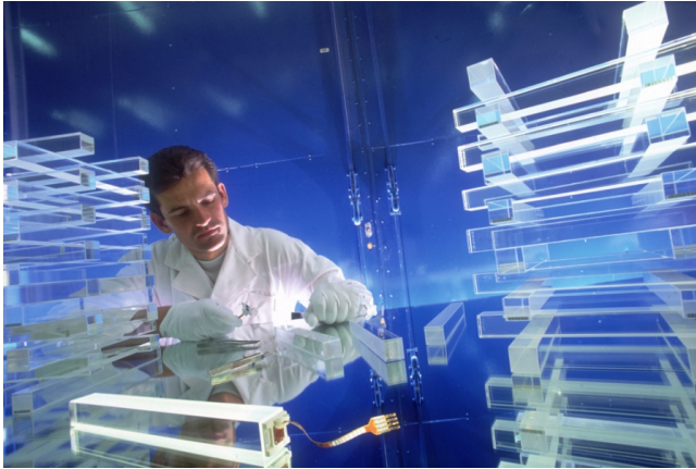
Figure 17.15: Preparation of the \text{PbWO}_4 single crystal scintillators for CMS. The electromagnetic calorimeter of CMS consists of 75,848 such crystals read by avalanche photo-diodes
