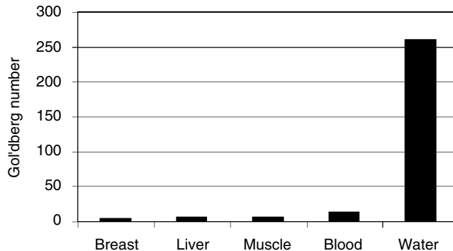
Figure 12.8 Gol'dberg numbers for tissue and water for a pressure of 5 MPa and a frequency of 5 MHz (from Szabo et al. , 1999, with permission from the American Institute of Ultrasound in Medicine).
