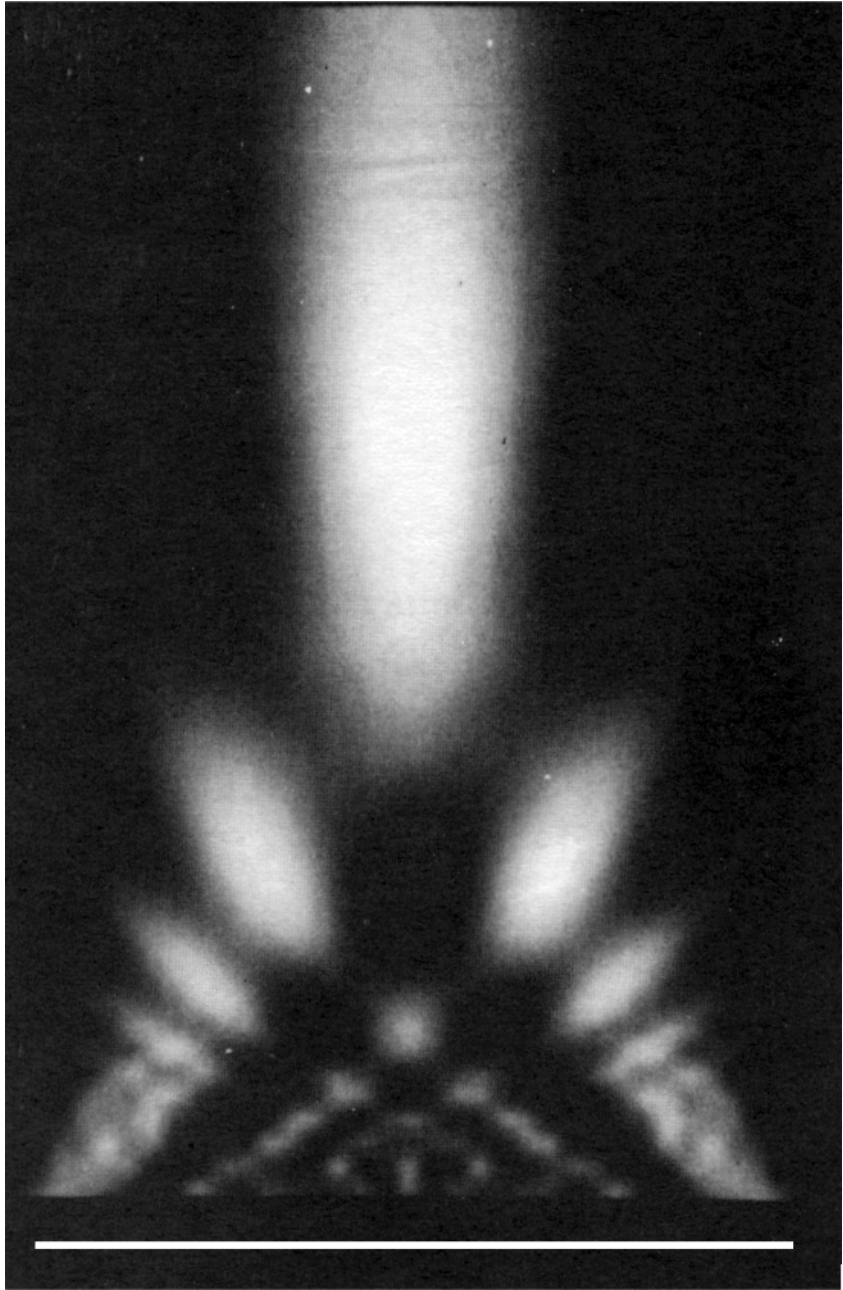
Figure 6.2 Top view of a diffracted field from a 40-wavelength-wide line aperture on the left. The same field from Figure 6.1 is shown in gray scale. The beam axis is compressed relative to the lateral dimension (from Szabo and Slobodnik, 1973).
