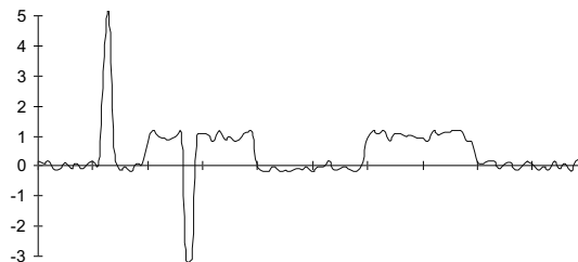
Input signal x(n) square wave with additive noise and impulsive noise transients.
