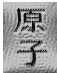
Fig. 4 Kanji character for "atom," by Lutz and Eigler, IBM, Almaden. An example of manipulation/mechanosynthesis of iron atoms on a Cu surface with an STM. (Courtesy of D. Eigler.)
