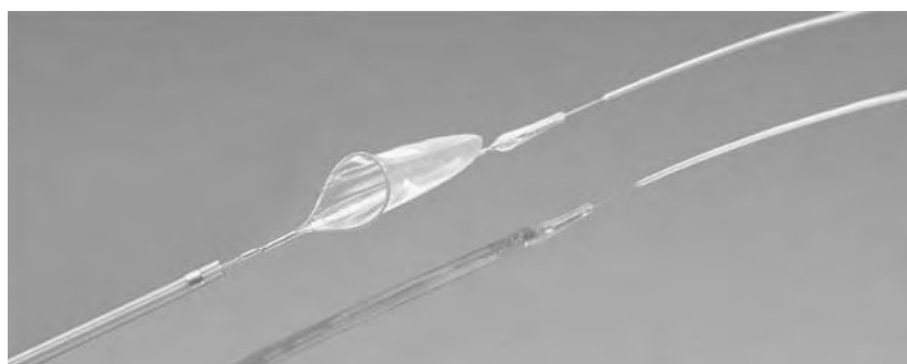
Fig. 4 The Filterwire EX of a nitinol filter loop mounted on a 0.014-inch guidewire. The filter material is made of polyurethane and has 80-micron pores to permit anterograde perfusion during deployment. The filter rotates freely on the end of the guidewire. The device is housed within a 1.3 mm (0.052 inch) delivery sheath. The loop has an off-center, fish-mouth design that facilitates complete apposition for vessels 3.5–5.5 mm in diameter. After the intervention, the device is retracted into the delivery sheath. The trapdoor action of the filter loop allows retention of the embolic debris during retrieval.
