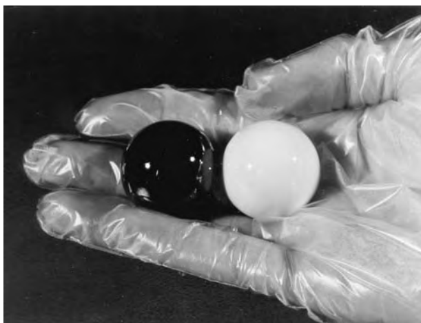
Fig. 3 DLC coated and uncoated alumina femoral heads.
