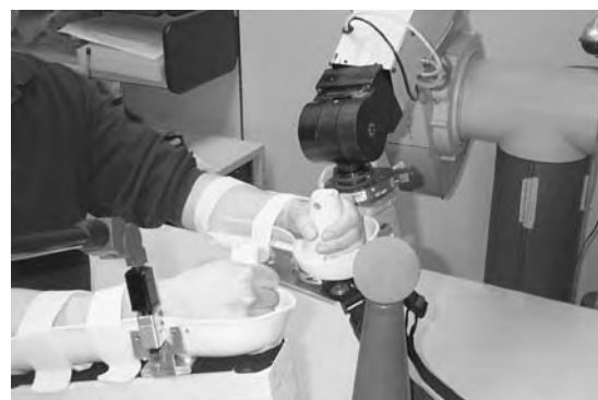
Fig. 3 Photograph of the MIME robotic system for delivering rehabilitation therapy to patients with arm impairment following stroke. (Photo courtesy of Peter Lum, Virginia Commonwealth University.)
