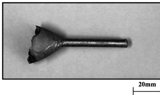
Fig. 18 Photograph of specimen of TNTZ cast using wax pattern formed with duplex coating of fine pure calcia and crushed silica fiber reinforced fine calcia.
