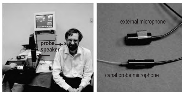
Fig. 5 A method of verifying the real ear gain of a hearing aid is depicted. An ear canal probe is placed between the eardrum and aid to measure the exact SPL. An external microphone provides the reference.
