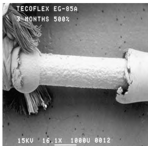
Fig. 7 Catastrophic failure: TecoFlex EG-85A, an aliphatic poly(ether)urethane. After three months, the tubing is seen fractured. A small piece of tubing still hangs on the left side of the mandrel, maintained in place by the left suture.
