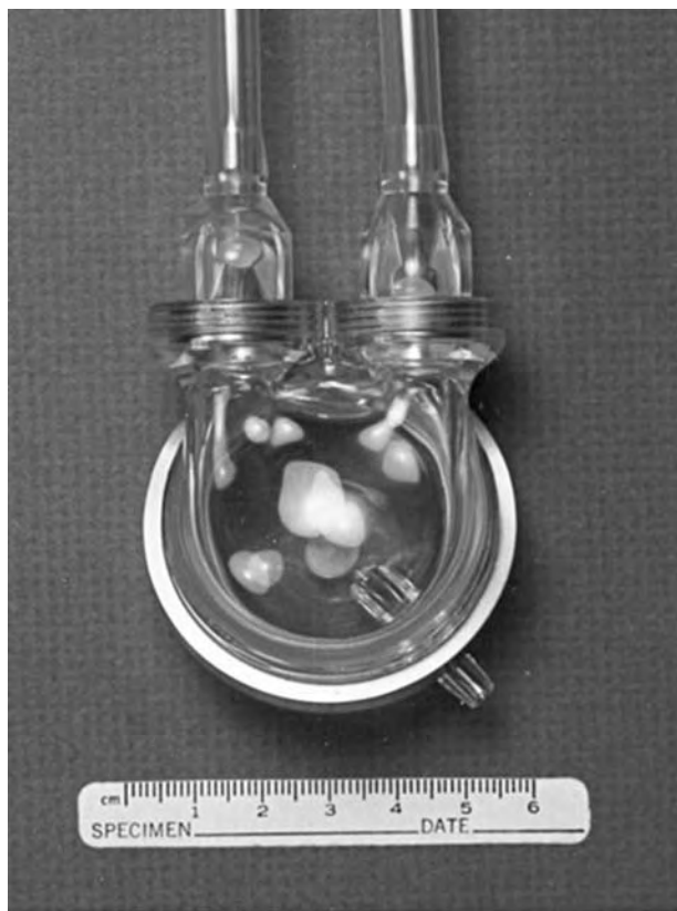
Fig. 4 The 15-cc Penn State pediatric ventricular assist device (circa 1995). The device measured 55 mm for the chamber outer diameter, 35 mm for the overall chamber thickness, 82 mm for the overall pump length with cannula connectors, and weighed 57 g.
