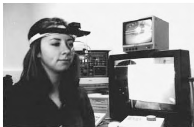
Fig. 2 A subject wearing a light, head-mounted eye tracker. The eye monitor, with crosshairs on the pupil and corneal reflection visible, is shown at the top right. The view from the scene camera, with the subject's point of gaze superimposed, can be seen at the bottom right.
