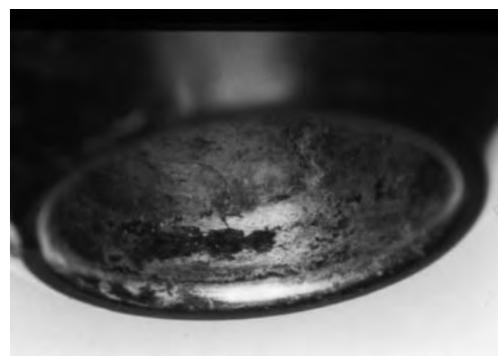
Fig. 4 Modular THA junction taper connection showing corrosion of taper connections. Macrograph of deposits of \text{CrPO}_4 corrosion particle products on rim of a modular cobalt-chrome femoral head.
