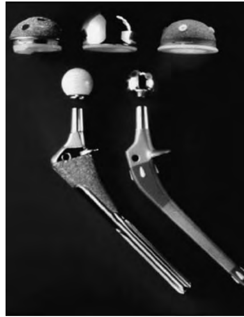
Fig. 2 Common type of total hip arthroplasty—titanium alloy stem, with cobalt-based alloy (ASTM F-75) modular head bearing on an ultrahigh molecular-weight polyethylene (UHMWPE) liner within a titanium alloy cup. Also shown is a ceramic head and three acetabular sockets with various surfaces for both cemented and cementless fixation. (Photograph courtesy of Zimmer, Inc.)
