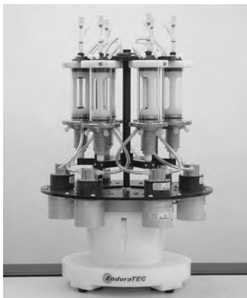
Fig. 8 Six-station BioReactor configuration showing individual chambers and mean pressure pumps.
