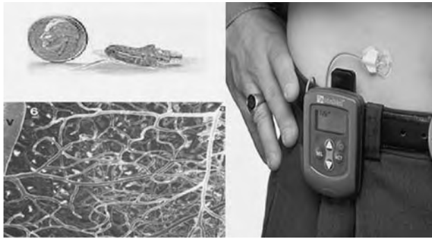
Fig. 3 Needle-type glucose sensor with arterioles, capillaries, and venules of subcutaneous tissue. The pictured sensor is manufactured by Medtronic-MiniMed as the Continuous Glucose Monitoring System-CGMS. (Used with permission from Medtronic-MiniMed Corporation, www.medtronic-minimed.com .)
