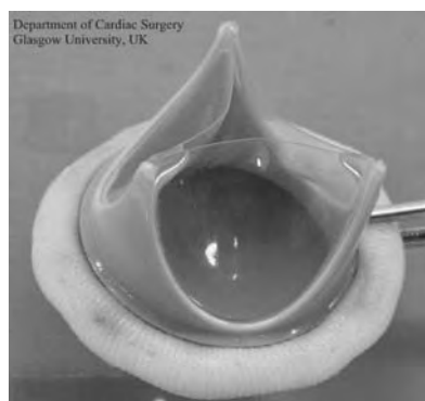
Fig. 4 PDMS-PU heart valve on a poly(etheretherketone) frame, sewing ring attached, explanted after six months, in the mitral position. (From Ref. [68].)
