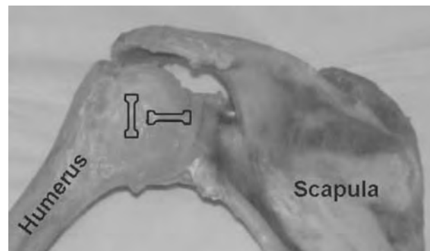
Fig. 5 View of the posterior capsule illustrating the orientation of the dog-bone-shaped (midsubstance 12.5 mm × 2.5 mm) transverse and longitudinal tissue samples with respect to the posterior band (PB-IGHL).
