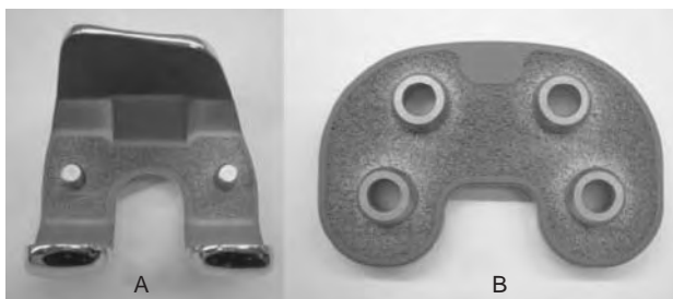
Fig. 1 Location of the (A) femoral and (B) tibial beaded component surfaces.
