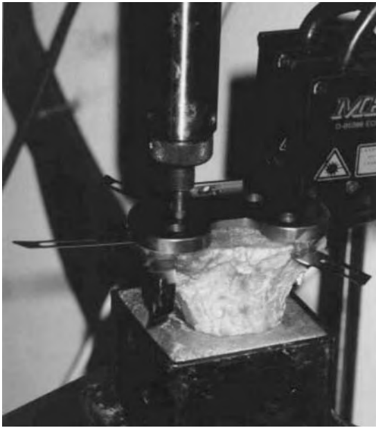
Fig. 3 Machine setup for testing tibial plate micromotion with four-screw fixation.
