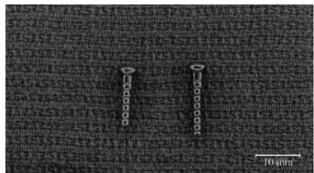
Fig. 14 Photograph of fractured screws.
