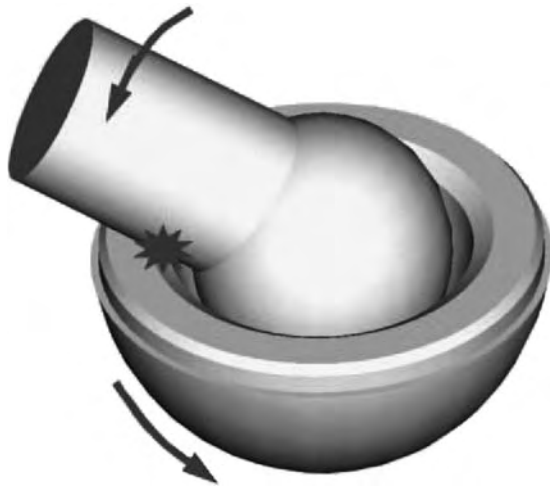
Fig. 4 An illustration of a femoral stem impinging on an acetabular cup.
