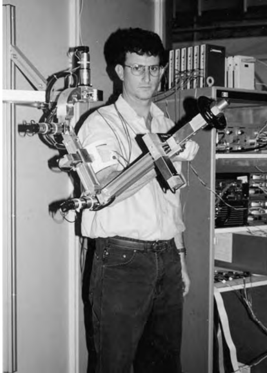
Fig. 2 Photograph of an exoskeleton for assisting arm movement under development at the University of Washington.
