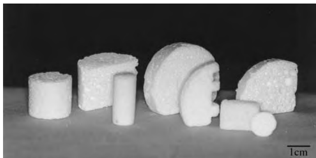
Fig. 3 Typical sol-gel-derived microporous scaffolds made in various shapes. (Picture courtesy of Dr. Pilar Sepulveda.)
