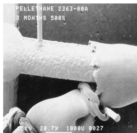
Fig. 8 Pellethane 2363-80A. After three months, this aromatic poly(ether)urethane has undergone complete failure, secondary to microcracking. This is classical environmental-stress cracking (ESC), which is followed by fracture.
