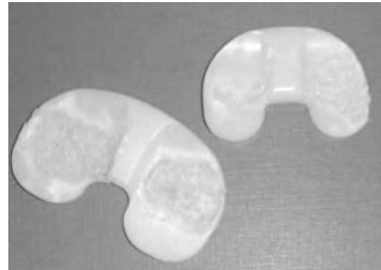
Fig. 4 Meniscal inserts demonstrating delamination.
