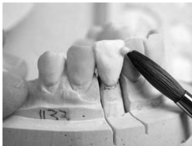
Fig. 5 Stacking feldspathic dental porcelain powder upon a die to form a dental crown.
