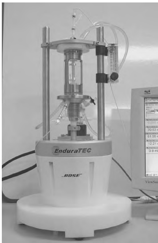
Fig. 6 Single-station BioReactor showing the moving magnet motor to provide dynamic pressure pulsing.
