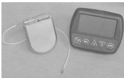
Fig. 6 Enzyme-based electrochemical/oxygen sensor for long-term implantation with the tip of the flexible lead (sensing region) free-floating in the superior vena cava. Intravenous (IV) sensor developed by Medtronic-MiniMed Corporation. (Used with permission from Medtronic-MiniMed Corporation, www.medtronic-minimed.com .)
