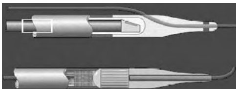
Fig. 2 Two types of IVUS catheters. The top drawing is a single rotating ultrasound element transducer and the lower drawing is of a solid-state ultrasound array transducer. (Reprinted with permission from Ref. [20]. © 1997 IEEE.)
