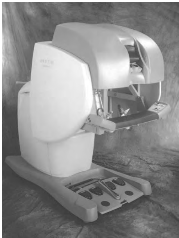
Fig. 2 The da Vinci control console at which the operating surgeon is seated.
