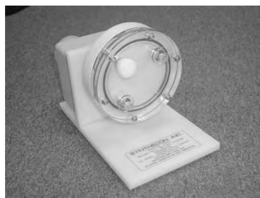
Fig. 3 The HARV. The vessel is disc-shaped and has a silicon membrane on the back. The gas mixture is pumped into the back of the vessel.
