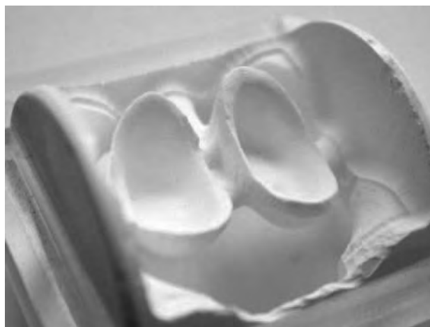
Fig. 9 Zirconia frameworks for porcelain crowns machined oversize by CAD–CAM (CERCON), prior to trimming and firing.
