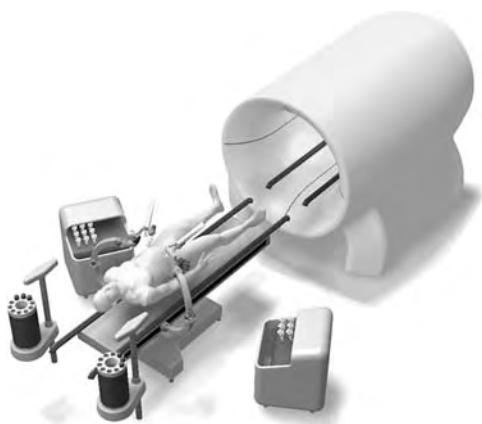
Fig. 7 A futuristic rendering of some of the subsystems that might be incorporated into the operating room of the future, including a modular operating table, surgical robotic arms, a tools changer, an equipment dispenser, and an imaging device.
