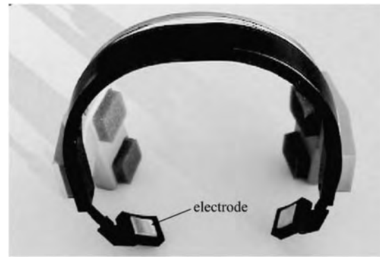
Fig. 1 Headset with electrodes for transdermal electrical stimulation for tinnitus treatment. High frequencies were modulated on an ultrasonic carrier with the device (Theraband) capacitive coupled to the head during stimulation.
