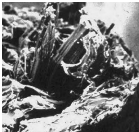
Fig. 1 Self-reinforcing structure is seen in an electron microscopy image. The long fibers are protruding out of the fractured surface of an SR-PLLA rod.
