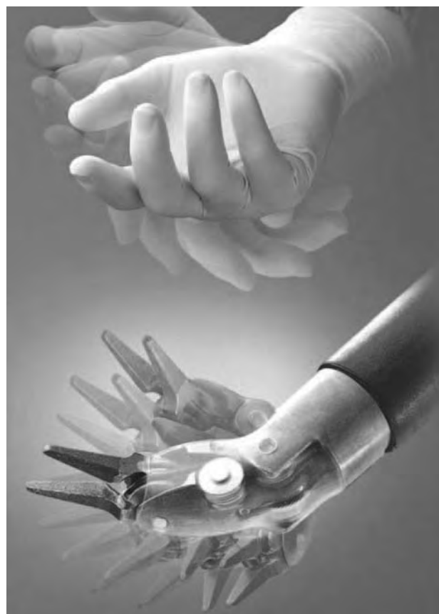
Fig. 1 A da Vinci intracorporeal operating instrument, illustrating the similar range of motion and DOF with the surgeon's hand.
