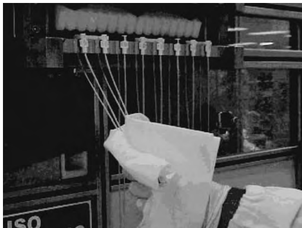
Fig. 7 Photograph illustrating the process of wiping the catheter surface following dipping in MDX4-4159 fluid. (Courtesy of Cordis de Mexico S.A. de C.V., Chihuahua, Mexico.)
