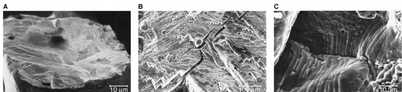
Fig. 32 (A) SEM micrograph of fracture surface of Co–Cr–Mo hip stem; (B) SEM micrograph showing saw tooth pattern on fracture surface indicative of Stage I fatigue crack growth; and (C) SEM micrograph showing fatigue striations and secondary cracking on fracture surface.
