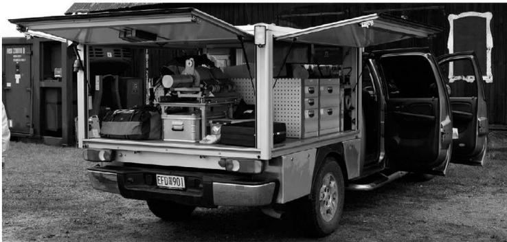
FIGURE 7.68 (a) Schematics view of the components used in a mobile gamma survey system. (b) Car-borne mobile  $\gamma$  survey system, with detector units mounted on a “cargo”.
