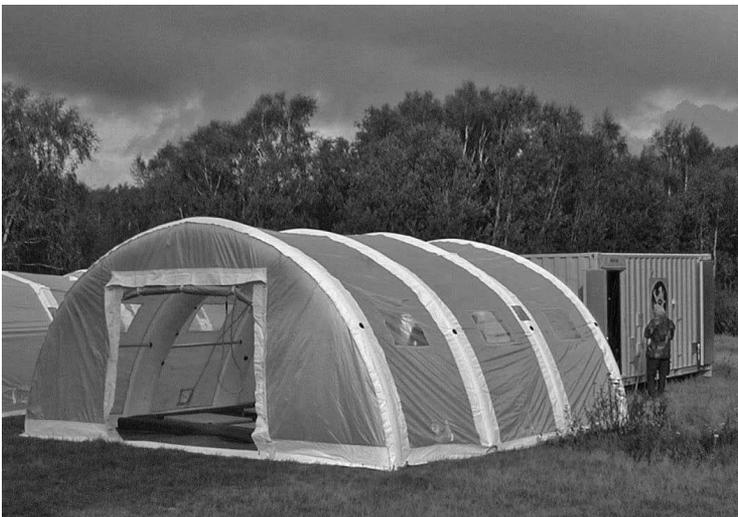
FIGURE 7.78 A decontamination unit providing complete decontamination of individuals exposed to hazardous substances such as chemicals and radioactive materials (photograph by R. Finck).
