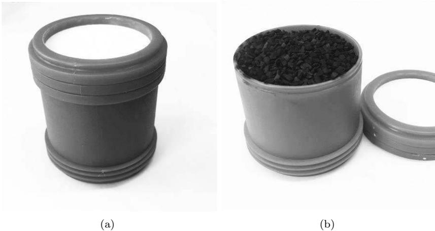
FIGURE 5.5 A typical air filter used in the Swedish emergency preparedness system for air sampling. The air filter is composed of a particle filter on top (a), and a charcoal column behind the particle filter (b).
