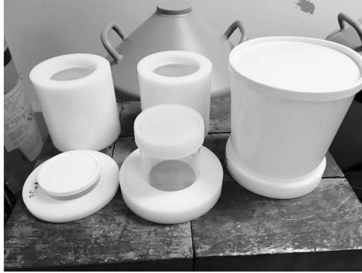
FIGURE 5.20 Standard beakers and sample holder geometries used for high-resolution  $\gamma$ -ray spectrometry.
