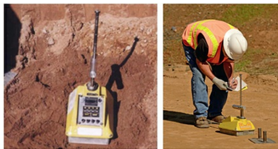
FIGURE 14.4 Moisture density gauges, used in the laying of tarmacadam road surfaces, contain small quantities of both americium-241 and cesium-137. About 22,000 are in use in the United States, and 50 or more are reported lost or missing each year. This material would be suitable to construct a “dirty bomb.” (Shutterstock/TFoxFoto)
