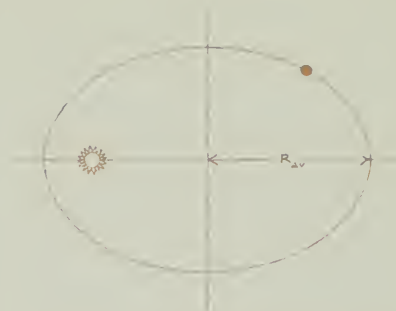
The value of R_{av} for an ellipse is just half the major axis.
