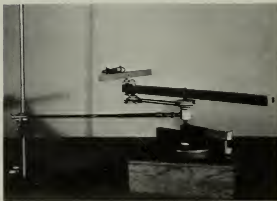
Fig. 5-15 An epicycle demonstrator connected to a turntable.
