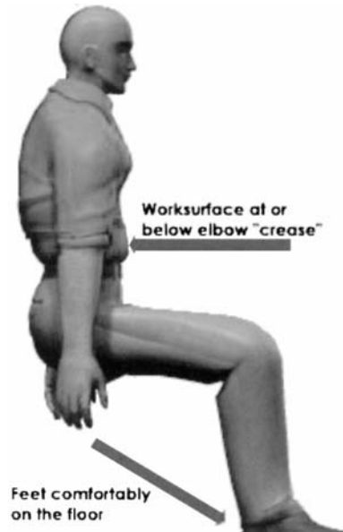
FIGURE 14.11 Body Reference Point for Worksurface Height.
