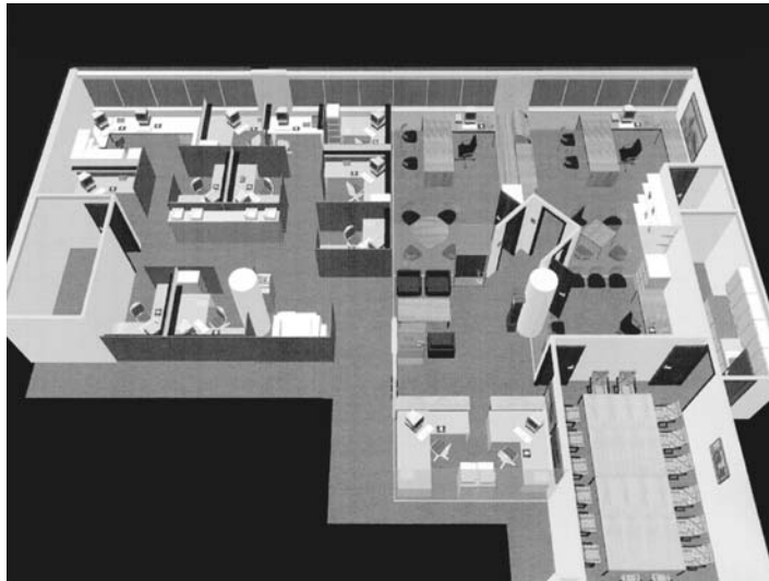
FIGURE 31.12 3D Visualization with User-Controlled Walk-Through Created with 3D CAD. (Source: Concept CAD reproduced with the permission of the Virtus Corporation.)
