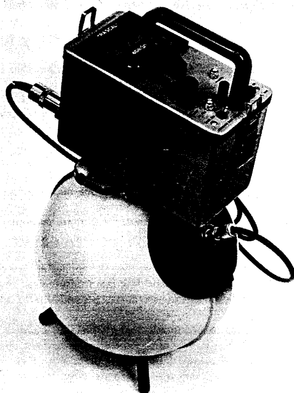
FIG. 16.5. A portable neutron rem counter, "Rascal." (Courtesy of Eberline, Santa Fe, NM.)
