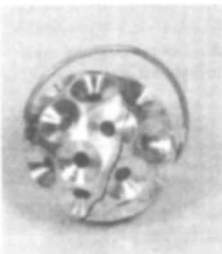
FIGURE 11.7. A perforated filter to reduce the photoelectric overresponse of a dosimeter while retaining response to photons below \cong 80 keV. The spherical design minimizes directional dependence. (Maushart and Piesch, 1967. Courtesy of R. Maushart.)
