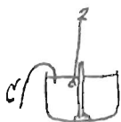
From Faraday's diary, a wire rotating around a magnet
