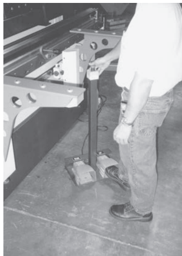
FIGURE 14-8 In order for this shearing machine to cut, both the foot pedal and the hand button must be engaged.
