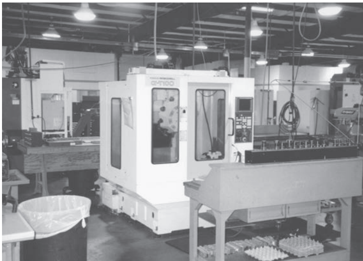
FIGURE 14-10 The safety door on this drilling machine must be closed or the drill will not operate.
