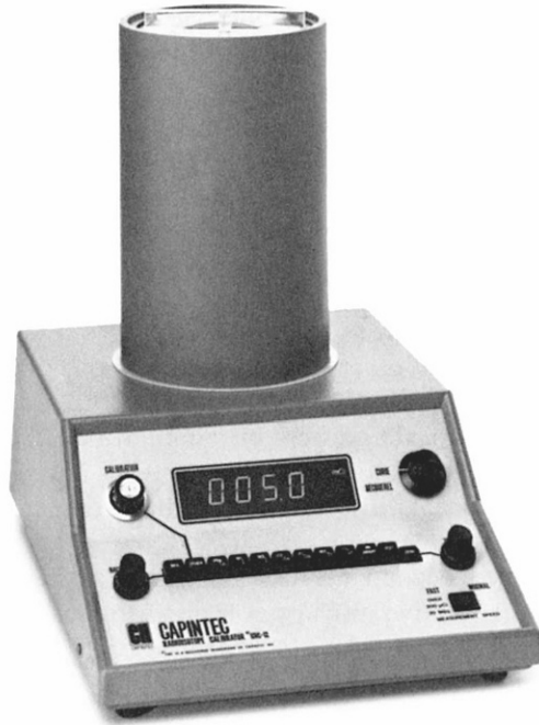
FIG. 7.3. A typical dose calibrator. (Courtesy of Capintec, Inc., Ramsey, NJ.)
