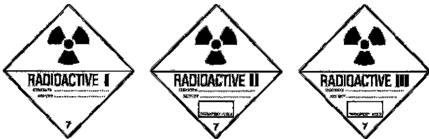
FIG. 16.3. The three types of U.S. Department of Transportation labels required for transportation of radioactive materials.
