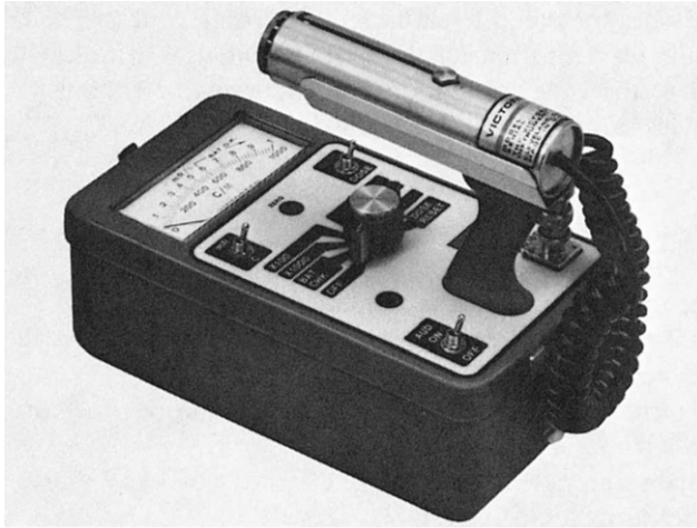
FIG. 7.4. An end-window-type Geiger-Müller counter. (Courtesy of Nuclear Associates, Carle Place, NY.)
